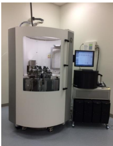
Figure 1.5. The SPINLab DNP polarizer at the UT Southwestern Medical Center for clinical applications. The DNP polarizer is shown on the left while the computer and quality control unit is on the right.
