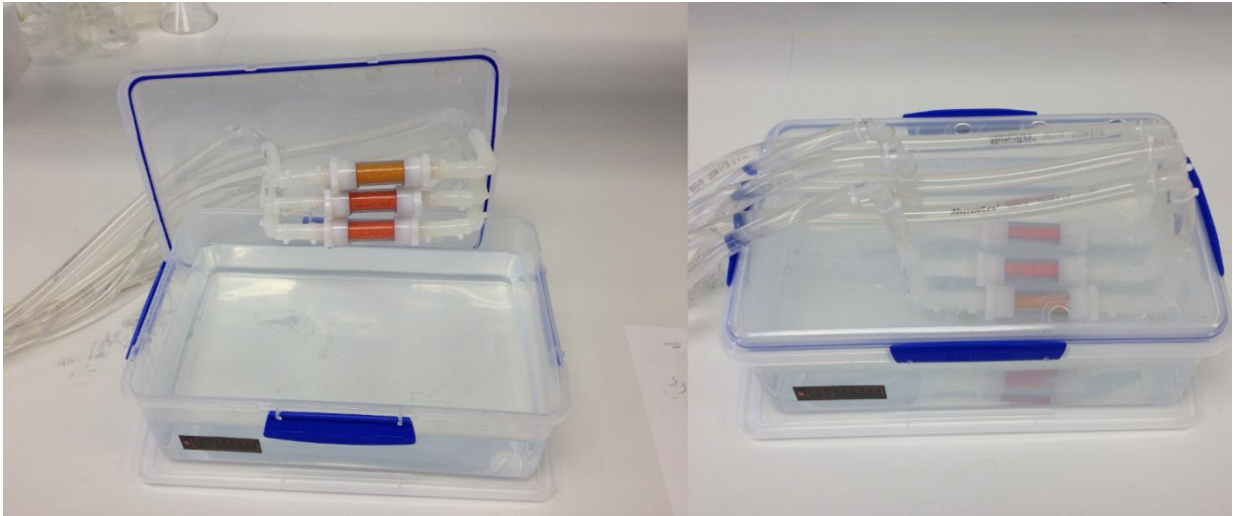
Figure 7.1: Original phantom design with three sponges in line with the tubing submerged in a water bath.
