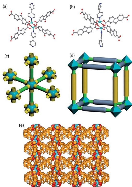
Fig. 1 SBUs of (a) LMOF-201 and (b) LMOF-202; Illustrations of (c) the connectivity of ligands (green) to the Zn core (aqua) and (d) a single cage of the framework; (e) The overall 3D structure of LMOF-202, viewed along the *a* axis. Colour code: white (H), orange (C), blue (N), red (O), aqua (Zn).
