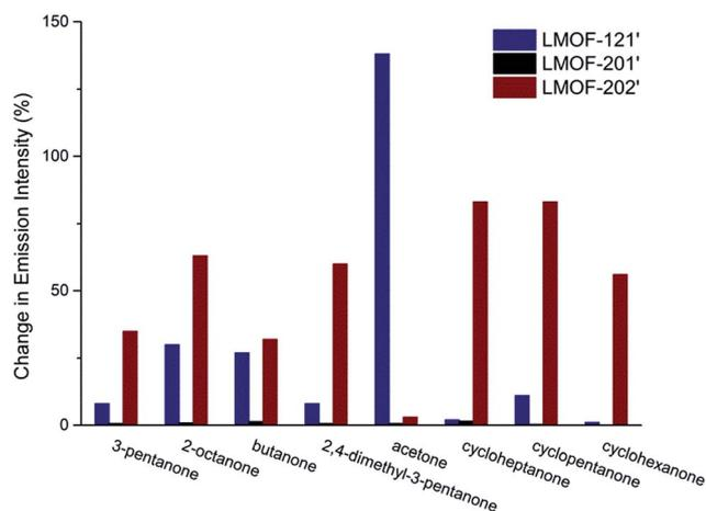
Fig. 2 A comparison of fluorescence enhancement after 10 s exposure of LMOF-121' and LMOF-202' to the vapors of ketones.
