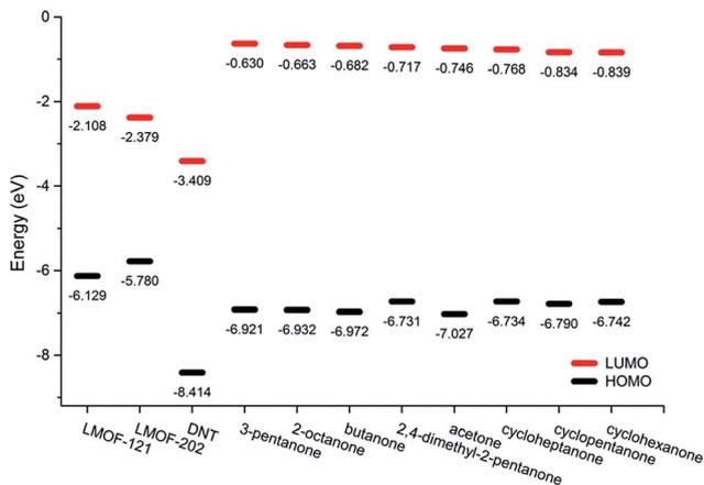
Fig. 4 An illustration of molecular orbital energy levels of LMOF-121, LMOF-202, and analytes computed at B3LYP/SDD (on Zn), 6-31+G\*(on H, C, N, O).<sup>41</sup>
