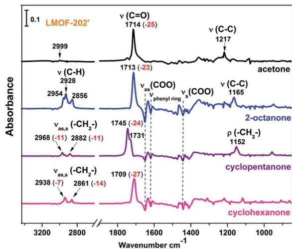
Fig. 5 IR absorption spectra of adsorbed ketone molecules: acetone, 2-octanone, cyclopentanone, cyclohexanone in LMOF-202' referenced to IR spectrum of blank LMOF-202'. The spectra were recorded after exposing LMOF samples to vapors for 3 min.
