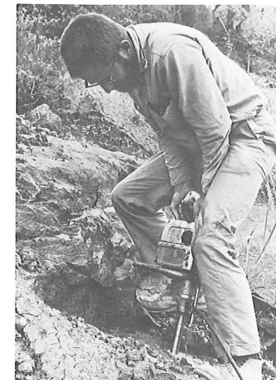
Dr. Charles E. Helsley uses a core drill to take a rock sample for magnetic studies.
