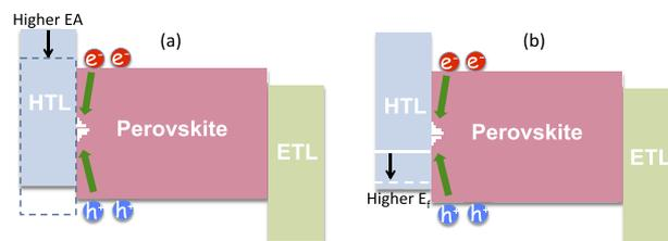
FIG. 1. Schematic of the device structure used in our simulations. The HTL electronic level position is varied through (a) varying the HTL EA while keeping  $E_g$  unchanged and (b) varying the HTL  $E_f$  through dopant concentration ( $N_A$ ). Green arrows indicate the interfacial recombination of electrons and holes through the defect states at the HTL-perovskite interface (short line at the interface).
