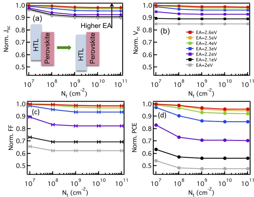
FIG. 4. Simulated  $J_{sc}$  (a),  $V_{oc}$  (b), FF (c), and PCE (d) for devices with different EA values for the HTL: 2.6 eV (red), 2.5 eV (orange), 2.4 eV (green), 2.3 eV (blue), 2.2 eV (purple), 2.1 eV (black), and 2 eV (gray). The arrow indicates the direction of increasing EA, as depicted in the inset of (a) for the two extreme cases. All parameters are normalized to the values of devices without interfacial defects.
