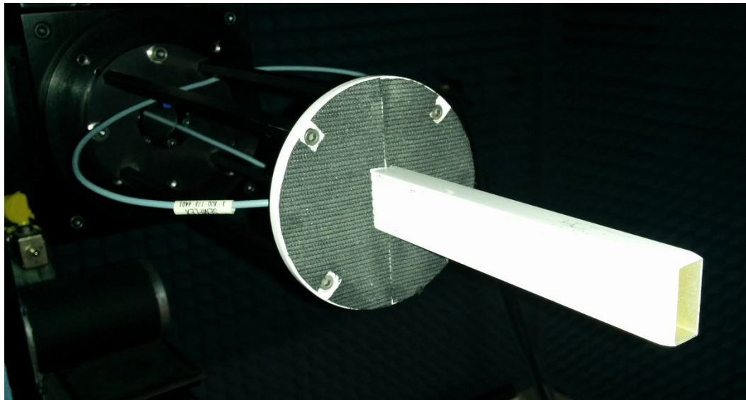
Figure F.3. Put the RF cable into the OEWG supporting structure.
