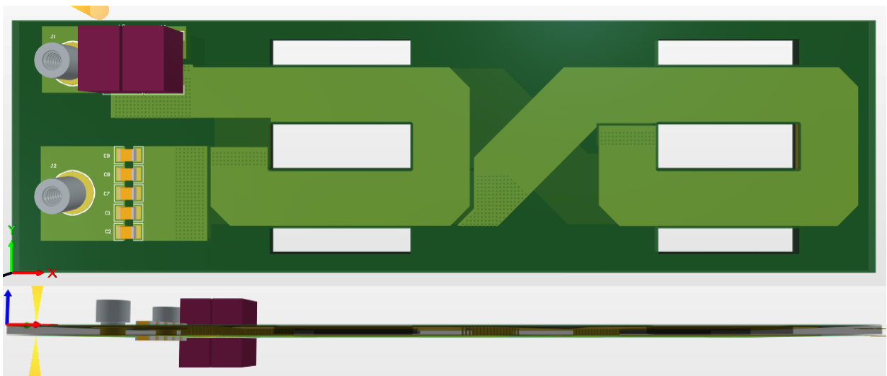
Figure 40: Top and side view of the LLC primary PCB
