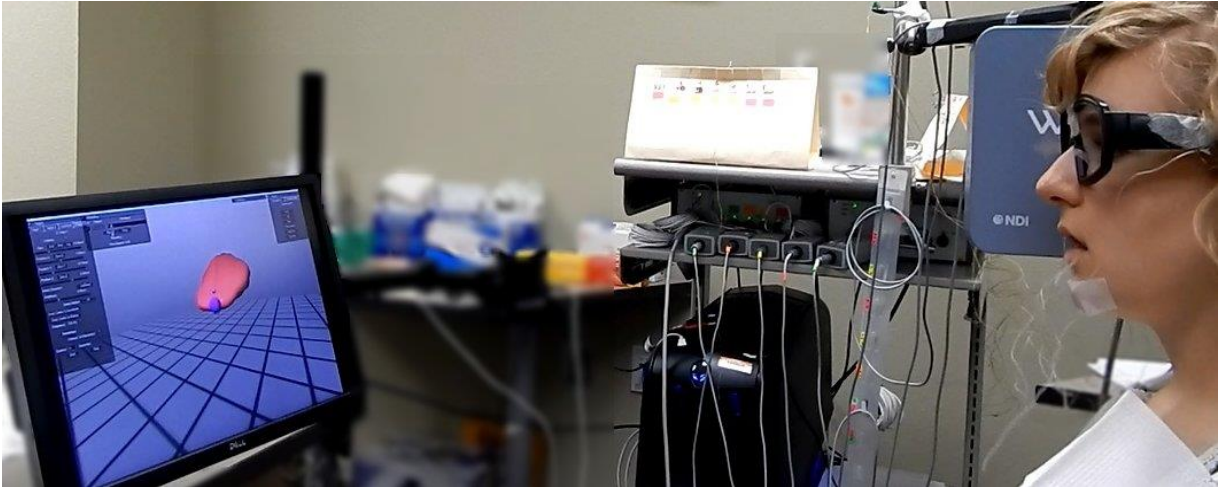
Figure C.1. Participant viewing tongue avatar, tongue tip marker, and oscillating target on computer monitor during tracking task.
