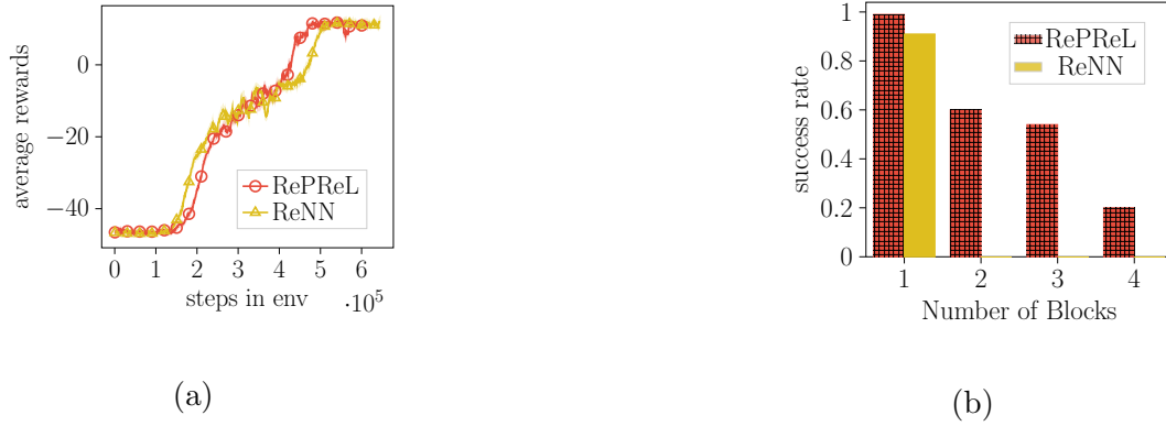
Figure 5.6: Comparing deep relational RL-based learners in FetchBlockConstruction. (a) Compares learning curve on the task of moving one block (b) Evaluates generalization for moving 1–4 blocks.
