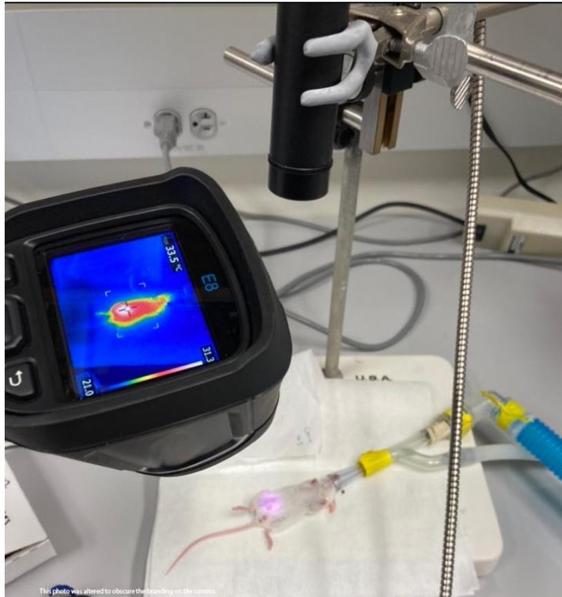
Figure A.1. Experimental setup consisting of a continuous 808 nm diode laser and a FLIR E6-XT thermal camera
