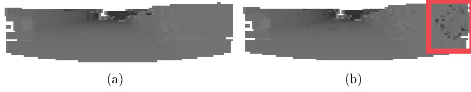
Figure 7.11: Failure case of cross-modal authentication: a) Depth map from LiDAR data, b) Depth map from stereo data (noisy region marked with the red rectangle).
