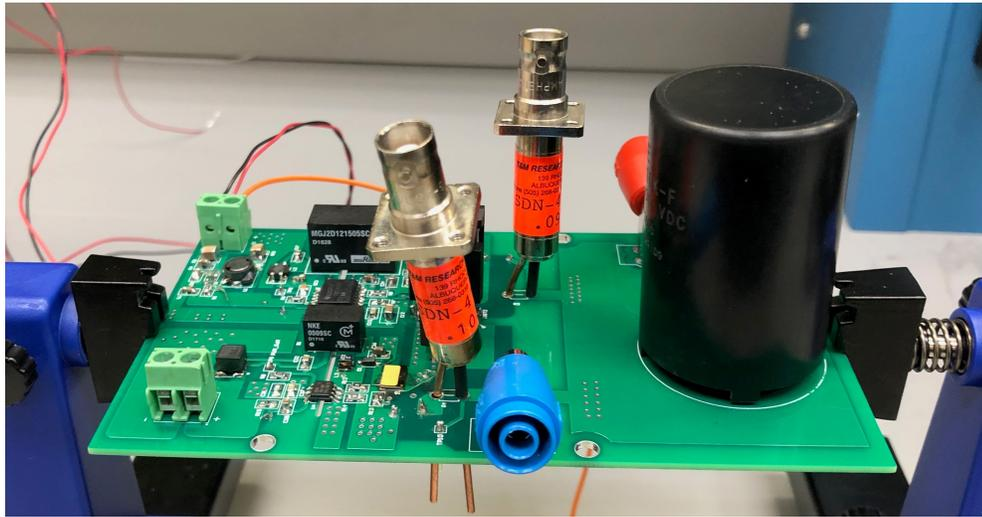
Figure A.4: DPT prototype for auxiliary inverter configuration side view
