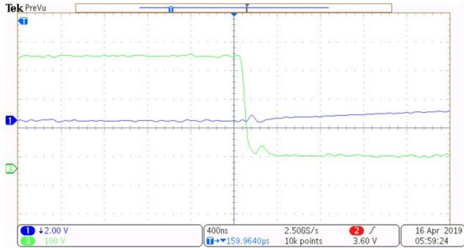
Figure 4.13: IGBT turn on waveform for 50A inductor current
