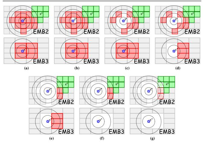
**Fig. 15** An idealised example of how the cell-by-cell subtraction works. Cells in two adjacent calorimeter layers (EMB2 and EMB3) are shown in *grey* if they are not in clusters, *red* if they belong to a  $\pi^+$  cluster and in *green* if contributed by a  $\pi^0$  meson. *Rings* are placed around the extrapolated track (represented by a *star*) and then the cells in these are removed ring by ring starting with the centre of the shower
