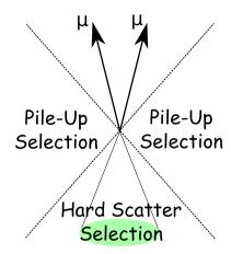
**Fig. 30** A diagram displaying the regions of  $r-\phi$  phase space which are expected to be dominated by hard-scatter jets (opposite in the  $r-\phi$  plane to the  $Z \to \mu\mu$  decay) and where there is greater sensitivity to pile-up jet activity (perpendicular to the  $Z \to \mu\mu$  decay)
