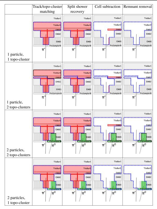
**Fig. 3** Idealised examples of how the algorithm is designed to deal with several different cases. The *red* cells are those which have energy from the  $\pi^+$ , the *green* cells energy from the photons from the  $\pi^0$  decay, the *dotted lines* represent the original topo-cluster boundaries with those outlined in *blue* having been matched by the algorithm to
