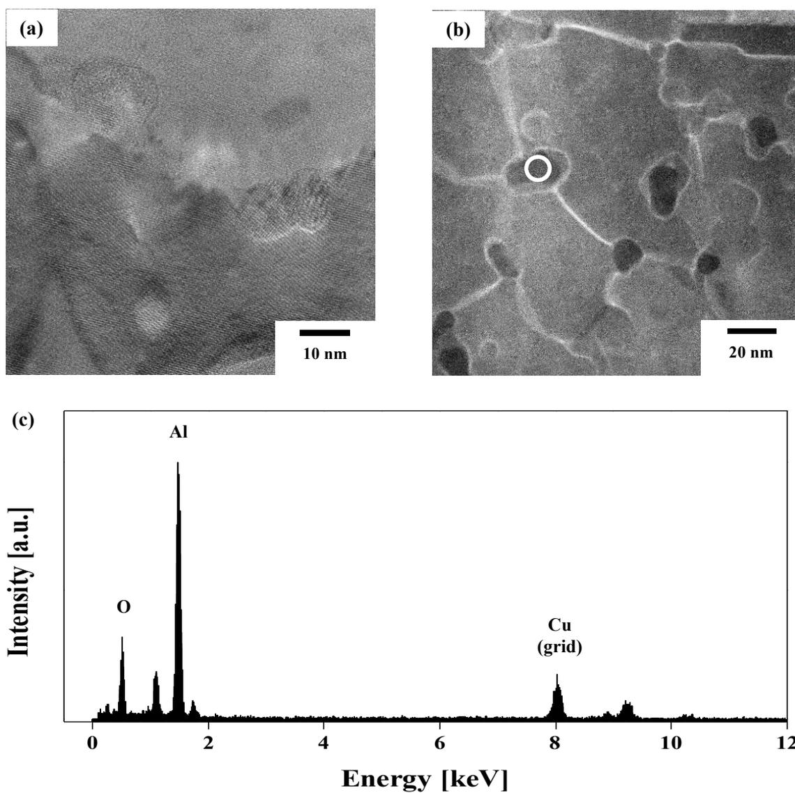
Supplementary Fig. S2 (a) TEM and (b) STEM-HAADF images of Al/BNNS composite after heat-treatment at 580 °C for 72 h. Supplementary Fig. 2 (c) shows EDS spectra, which is taken from the position marked with a white circle in (b).
