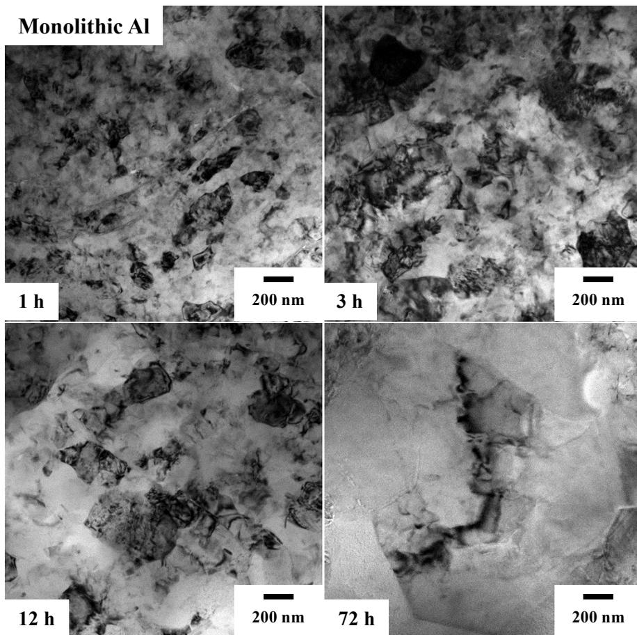
Supplementary Fig. S3 TEM images of monolithic Al after heat-treatment for 1, 3, 12, and 72 h.
