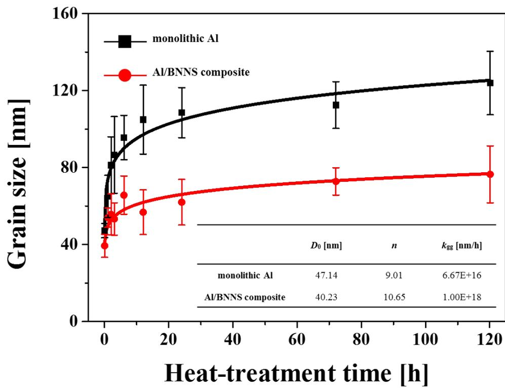
Supplementary Fig. S5 Grain size measured from XRD results and grain size evolution calculated by Eq. 2 with the calculated values in inserted table for monolithic Al and Al/BNNS composite after heat-treatment for varied times.
