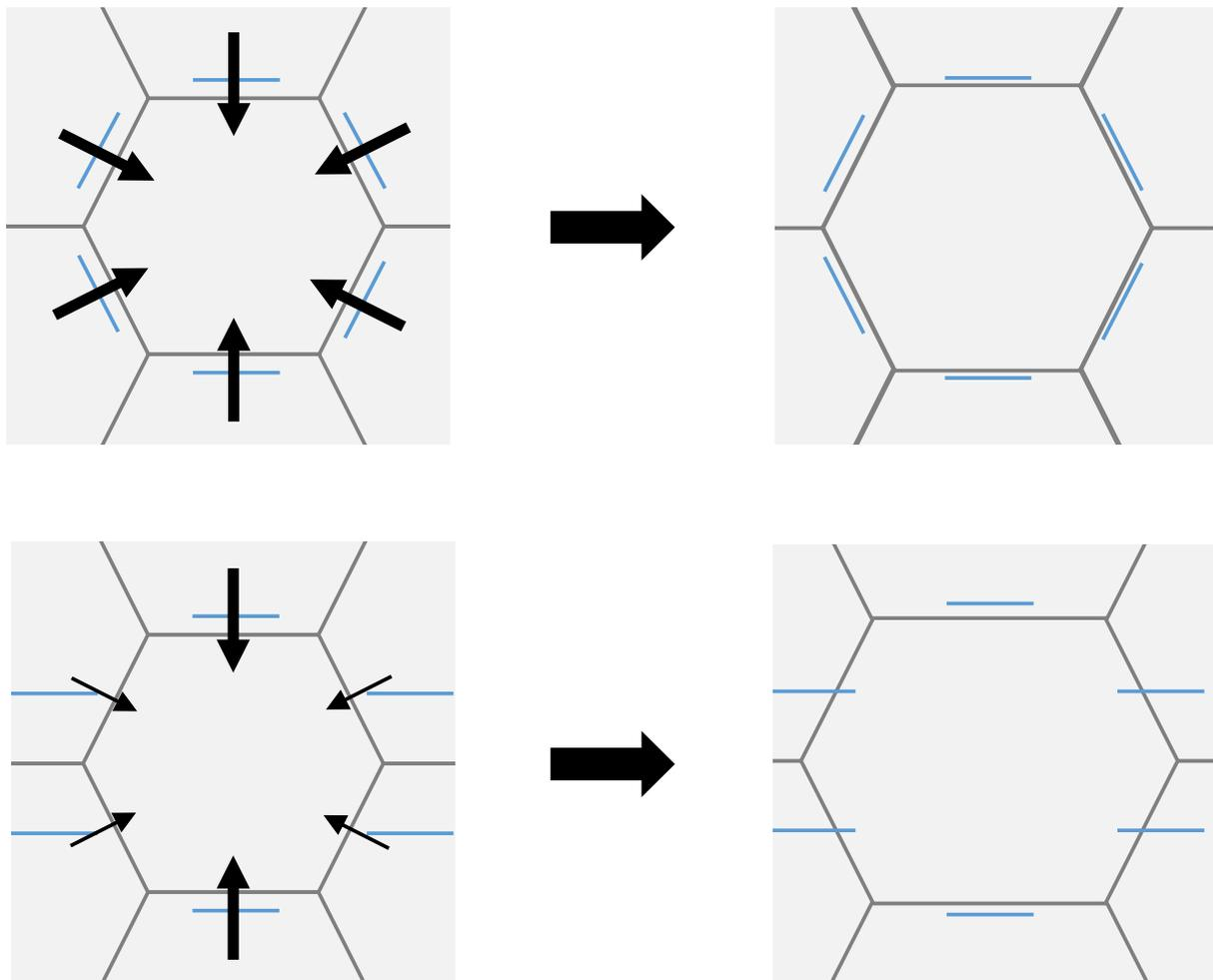
Supplementary Fig. S8 Schematic illustration of the grain growth behavior of randomly and unidirectionally oriented plate-like particle-containing composites. For the plate-like particles with random orientation with higher volume fractions, it is more likely that the grain boundary moves toward the normal direction of the particles.
