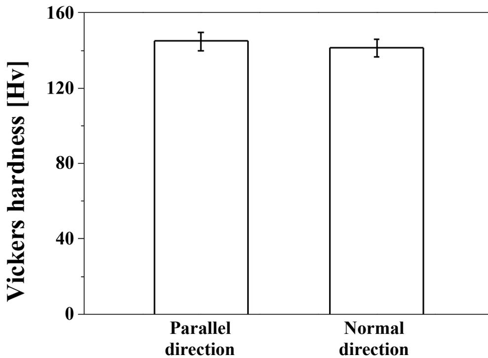
Supplementary Fig. S6 Vickers hardness for Al/BNNS composite measured on parallel and normal direction. The hardness measured parallel to the pressing direction is similar to that measured normal to the pressing direction. It means that the BNNS is dispersed in the Al matrix with random orientation.
