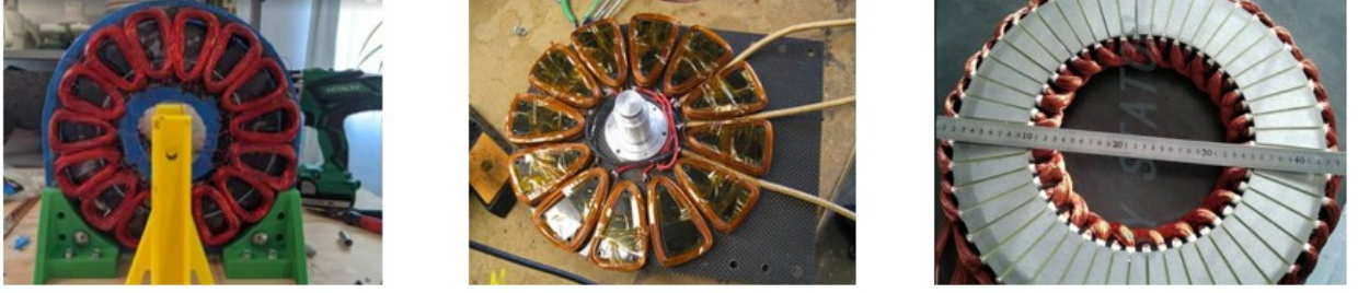
End windings of radial flux machine
