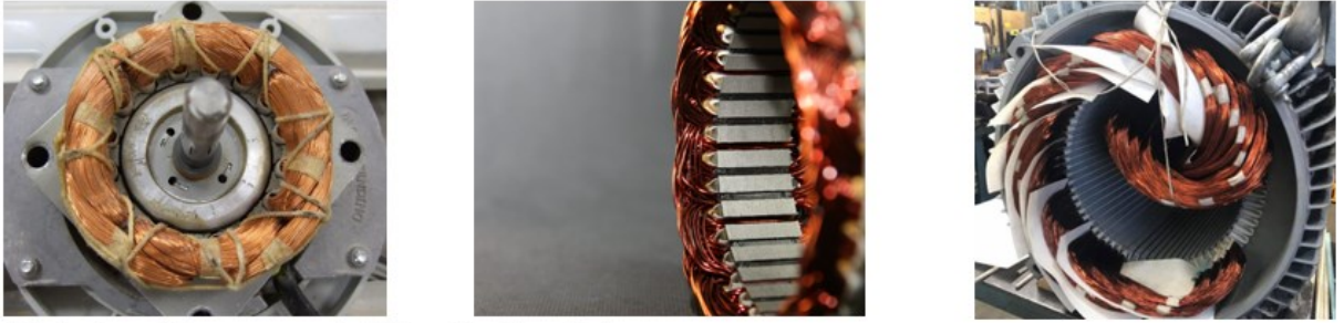
End windings of radial flux machine
