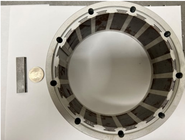
Figure 6.3: The rotor with installed rotor segments.
