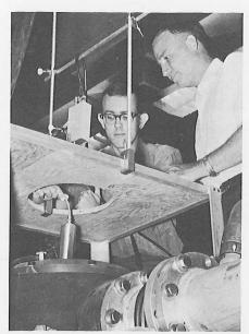
Professor Crawford and Steve Curry, graduate student, of Southern Methodist were first university users of the High Magnetic Field Facility. Mr. Curry is inserting a lithium-drifted silicon radiation detector and radiation source in the bore of the magnet, to determine effects on the detector.
