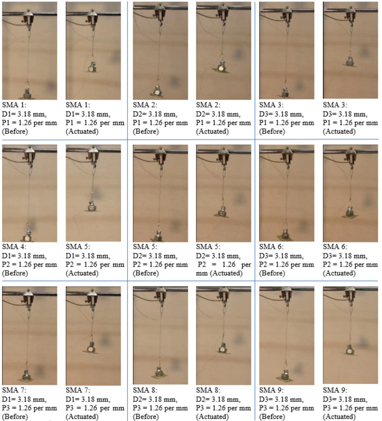
Figure 4.7. All 9 samples before actuation and after actuation.
