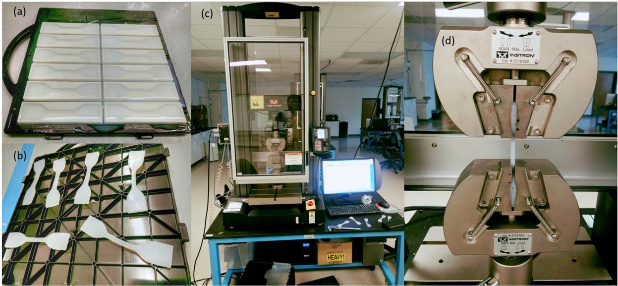
Figure 5.41. Tensile testing silicone (a) shows the ASTM D412 Type C 3D printed casings for Ecoflex-10 silicone casting, (b) the casted dog bone structures, (c) and (d) show the Instron tensile tester (maximum load 50 kN) machine with the silicone dog bone structure.
