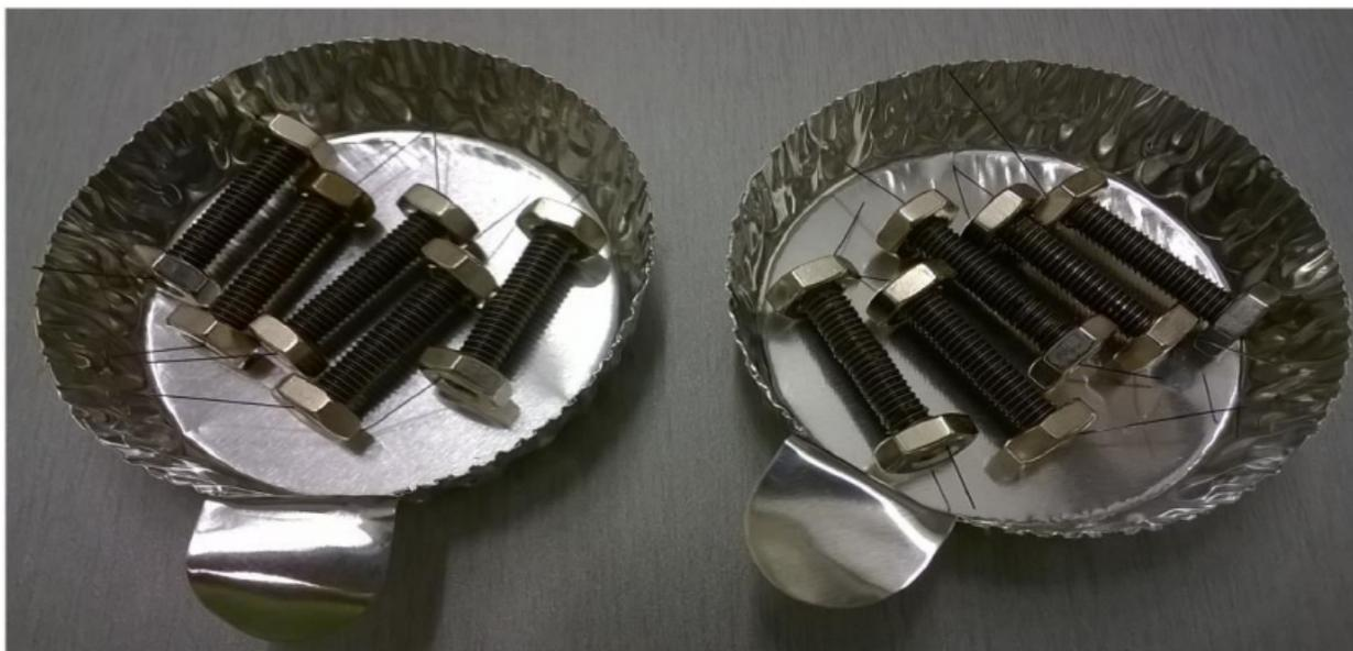
Figure 5.7. Fabrication of coiled SMA wires: SMA wires wrapped around bolts and secured by nuts .
