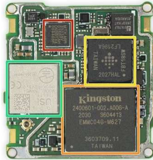
Figure 2.7. A motherboard of the Fitbit® Sense with a Mediatek® GPS SoC, Kingston® external flash memory, USI® BLE module, and FitBit® application SoC. Auxiliary sensors are on the other side of this board (not shown)[17].
