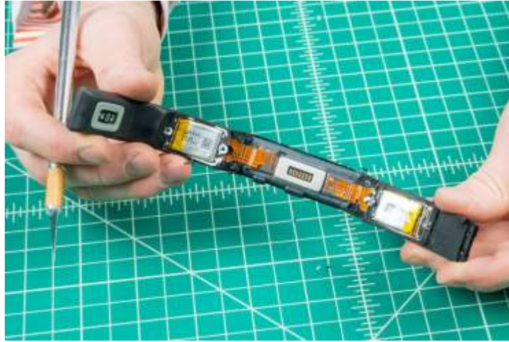
Figure 2.5. Teardown of a Microsoft® Band. The PPG sensor and the board are in the center of the band, whereas 2 batteries are integrated into the band body[15].
