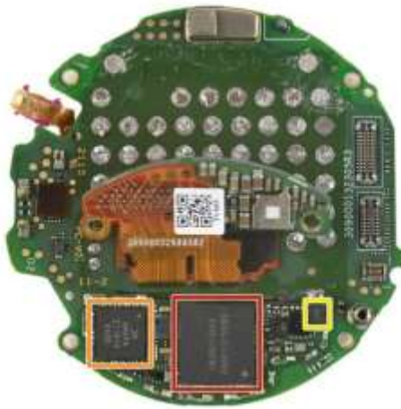
Figure 2.6. A motherboard of the Huawei® Watch 3 centered around Ambiq Apollo® 4 ARM® processor with an active current of 4\mu\text{A}/\text{MHz} . The recess above the processor is for the battery, whereas auxiliary circuits are on the other side of the board (not shown)[16].
