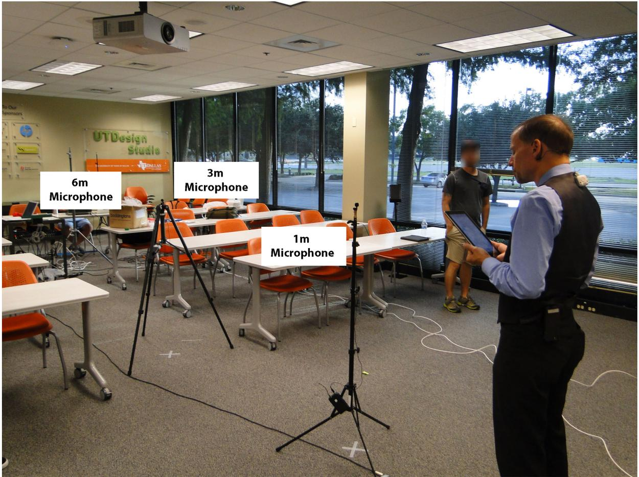
Figure 4.2. UTD-Distant Reverb Data Collection - Microphone and Speaker arrangement (Classroom)
