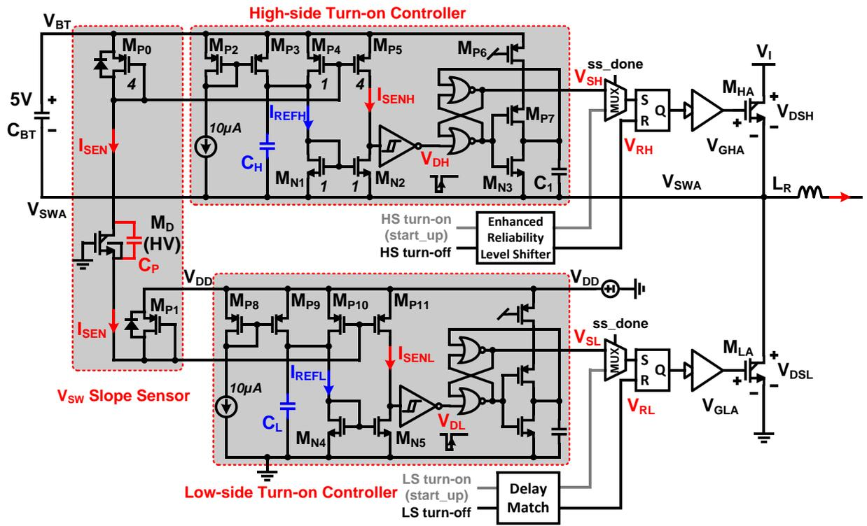
Figure 3.5. Schematic of the proposed SS-ZVSD.
