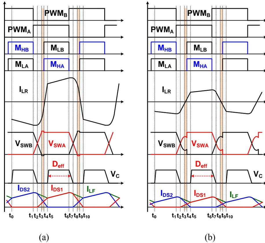
Figure 3.2. Key waveforms of (a) full-ZVS and (b) partial-ZVS operation of the proposed full-bridge converter.
