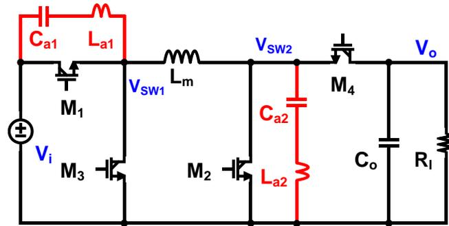
Figure 2.4. Schematic of QSW-ZVS non-inverting buck boost converter.
