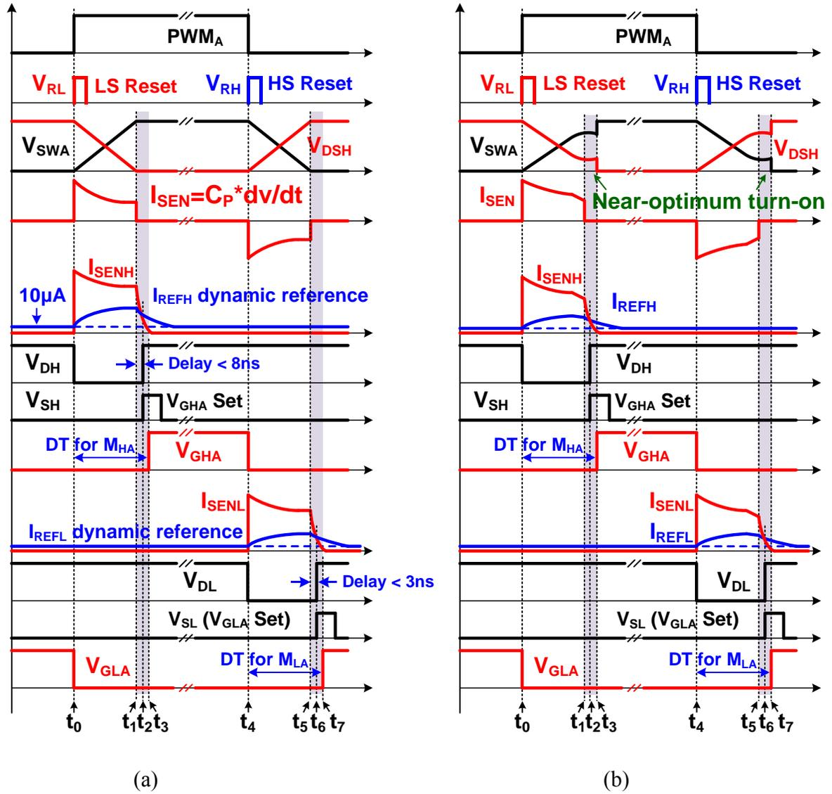
Figure 3.6. Timing waveforms of the SS-ZVSD during (a) full-ZVS and (b) partial-ZVS operations.
