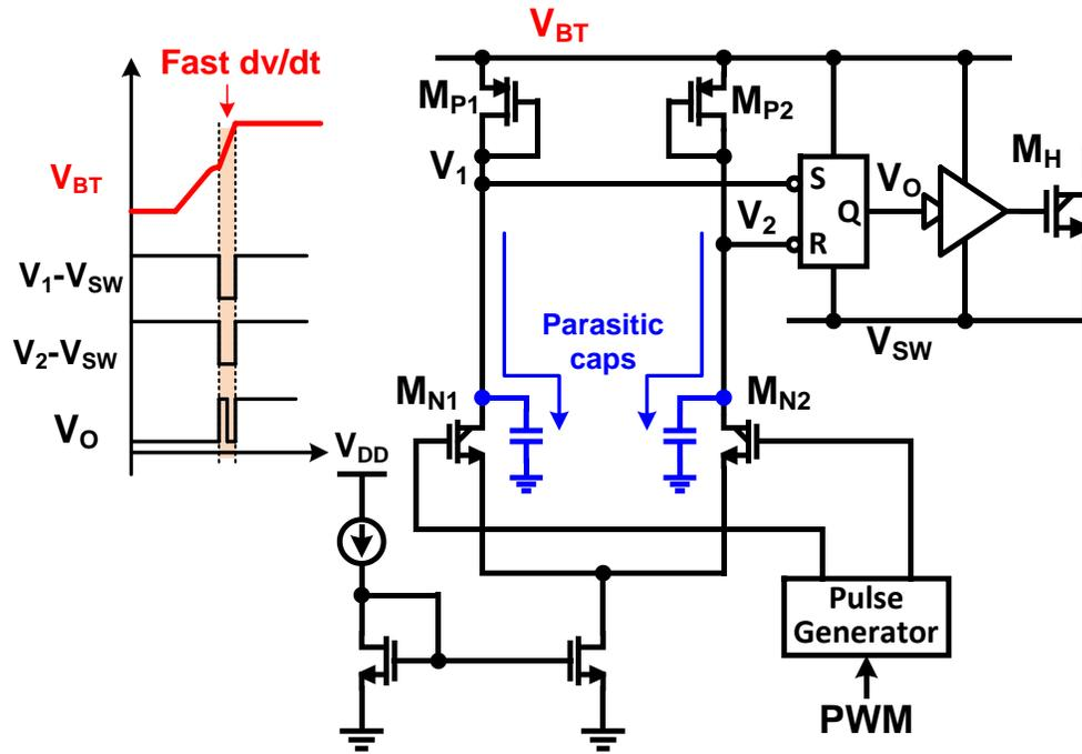
Figure 3.7. Structure and waveforms of a traditional HV level shifter.
