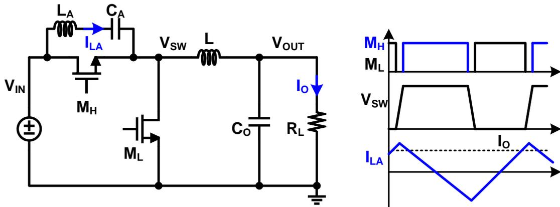
Figure 1.5. Schematic and waveforms of a conventional quasi-square-wave buck converter.
