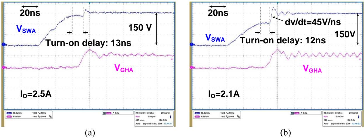
Figure 3.12. Measured  $t_{\text{total\_delay}}$  in partial-ZVS operation for (a)  $I_O = 2.5\text{ A}$  and (b)  $I_O = 2.1\text{ A}$ .
