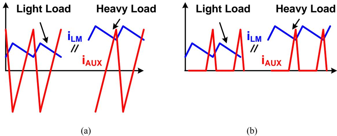
Figure 2.5. (a) Inductor waveforms of QSW-ZVS converters; (b) Inductor waveforms of ZVT converters.
