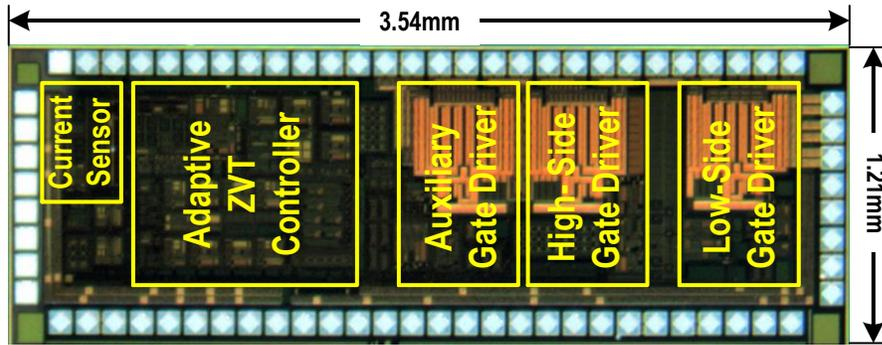
Figure 5.17. Micrograph of the proposed AZVT controller and converter gate driver in 0.5µm 120V CMOS process.
