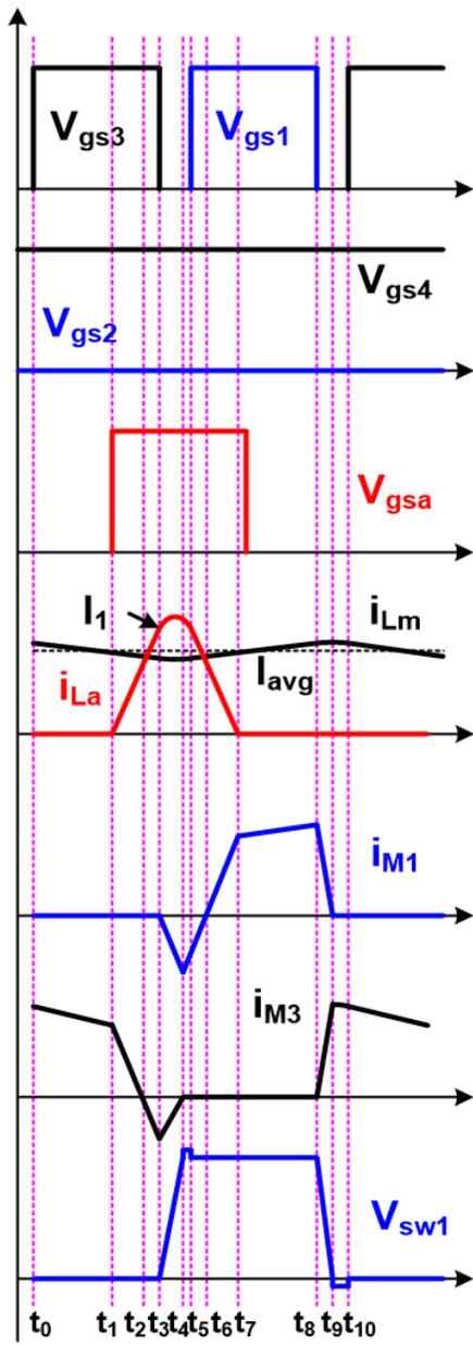
Figure 5.4. Key waveforms in the buck mode.
