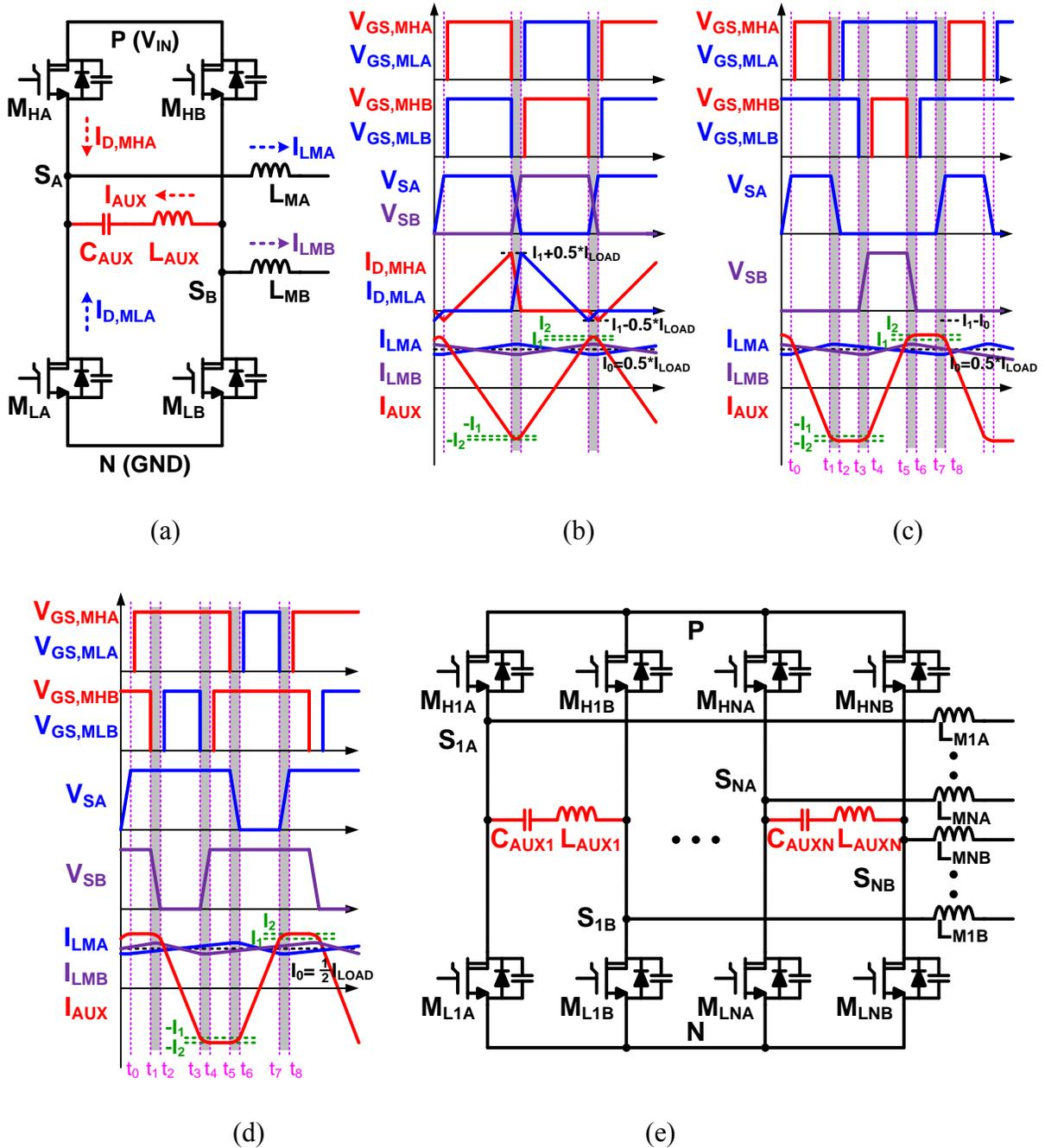
Figure 4.2. (a) Proposed PS-TPZVS cell; timing diagram of the PS-TPZVS cell under (b)  $D = 0.5$ , (c)  $D < 0.5$  and (d)  $D > 0.5$ ; and I 2N-phase PS-TPZVS cell.
