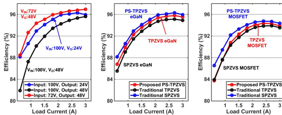
Figure 4.8. (a) Simulated power efficiency of the proposed converter vs load currents under different duty ratios (inductor core loss is included); and power efficiency comparisons among the proposed PS-TPZVS buck converter, the traditional single-phase ZVS converter, and the traditional two-phase ZVS converter under  $V_{IN} = 100\text{ V}$ ,  $V_O = 24\text{ V}$  with (b) eGaN FETs and (c) power MOSFETs.
