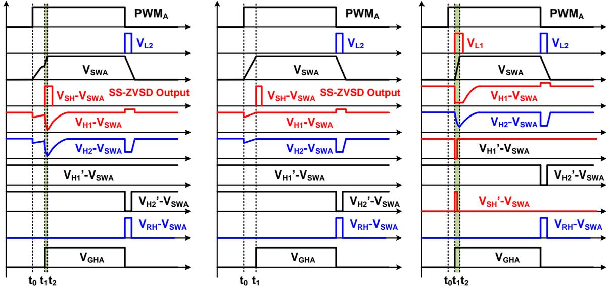
Figure 3.9. Operation waveforms of the proposed HV level shifter under (a) partial-ZVS, (b) full-ZVS, and (c) start-up conditions.
