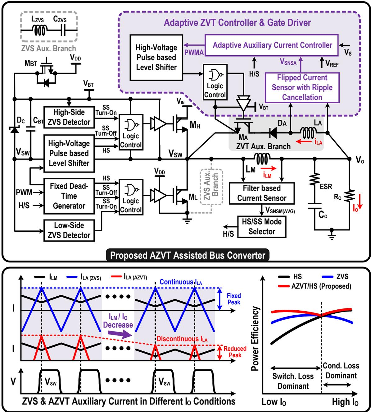
Figure 5.14. Structure of AZVT-assisted bus converter and comparison between AZVT vs ZVS in different load conditions.
