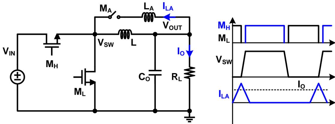
Figure 1.6. Schematic and waveforms of a conventional zero-voltage-switched buck converter.
