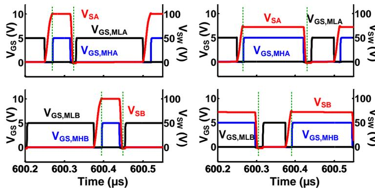
Figure 4.7. Simulated waveforms to demonstrate ZVS operation of the proposed converter under (a)  $V_{IN} = 100\text{ V}$ ,  $V_O = 24\text{ V}$ ,  $I_{OUT} = 3\text{ A}$ ; and (b)  $V_{IN} = 72\text{ V}$ ,  $V_O = 48\text{ V}$ ,  $I_{OUT} = 3\text{ A}$ .
