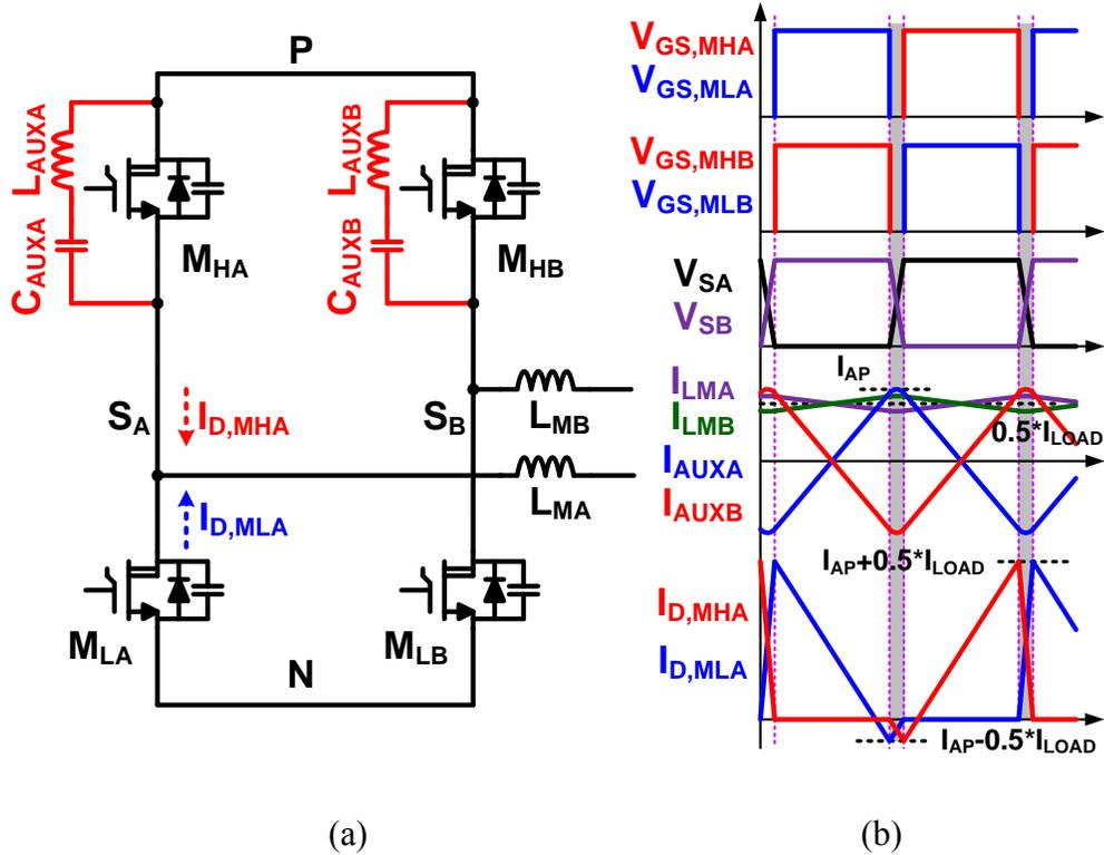
Figure 4.1. (a) structure and (b) timing diagram of a traditional two-phase ZVS cell.
