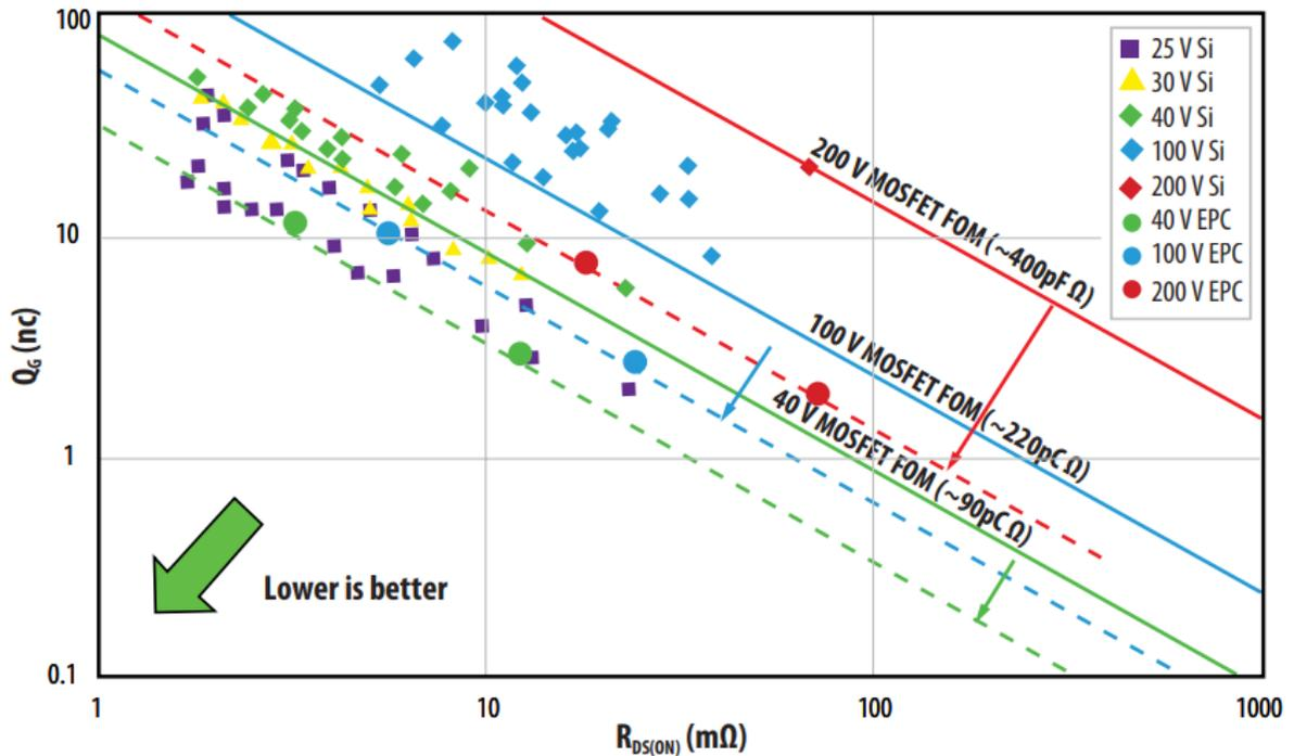
Figure 1.8. FoM comparison between GaN FETs and Si MOSFETs provided by EPC.
