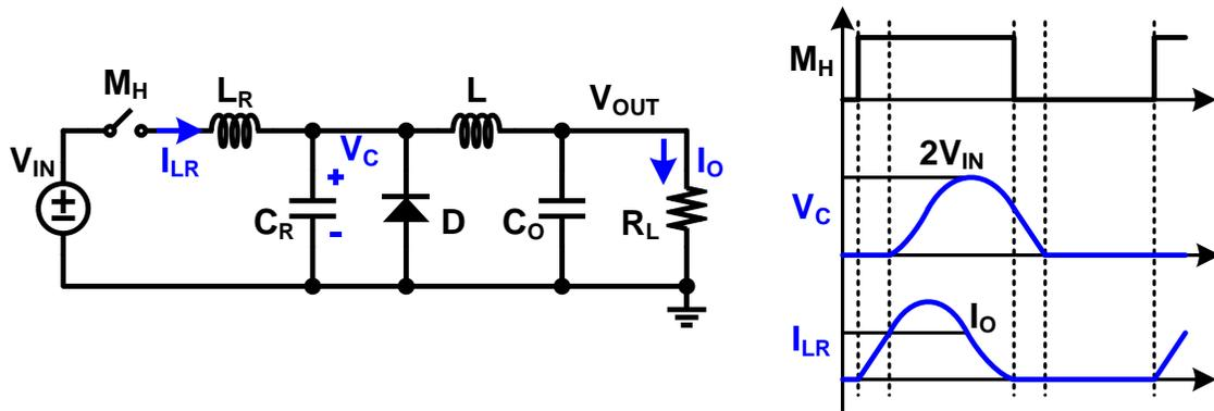
Figure 1.4. Schematic and waveforms of a conventional quasi-resonant buck converter.
