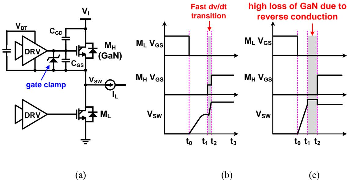
Figure 2.1. (a) Schematic showing design challenges of GaN drivers; (b) waveform of partial ZVS operation and (c) waveform of full ZVS operation.
