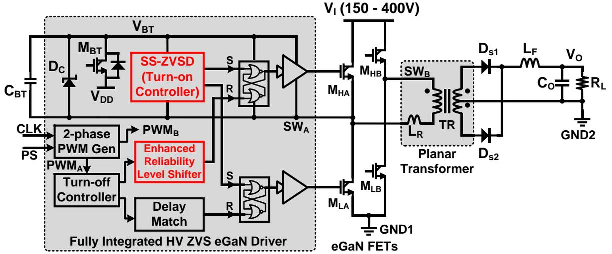
Figure 3.1. Schematic of the proposed isolated full-bridge bus converter with a monolithic ZVS driver.
