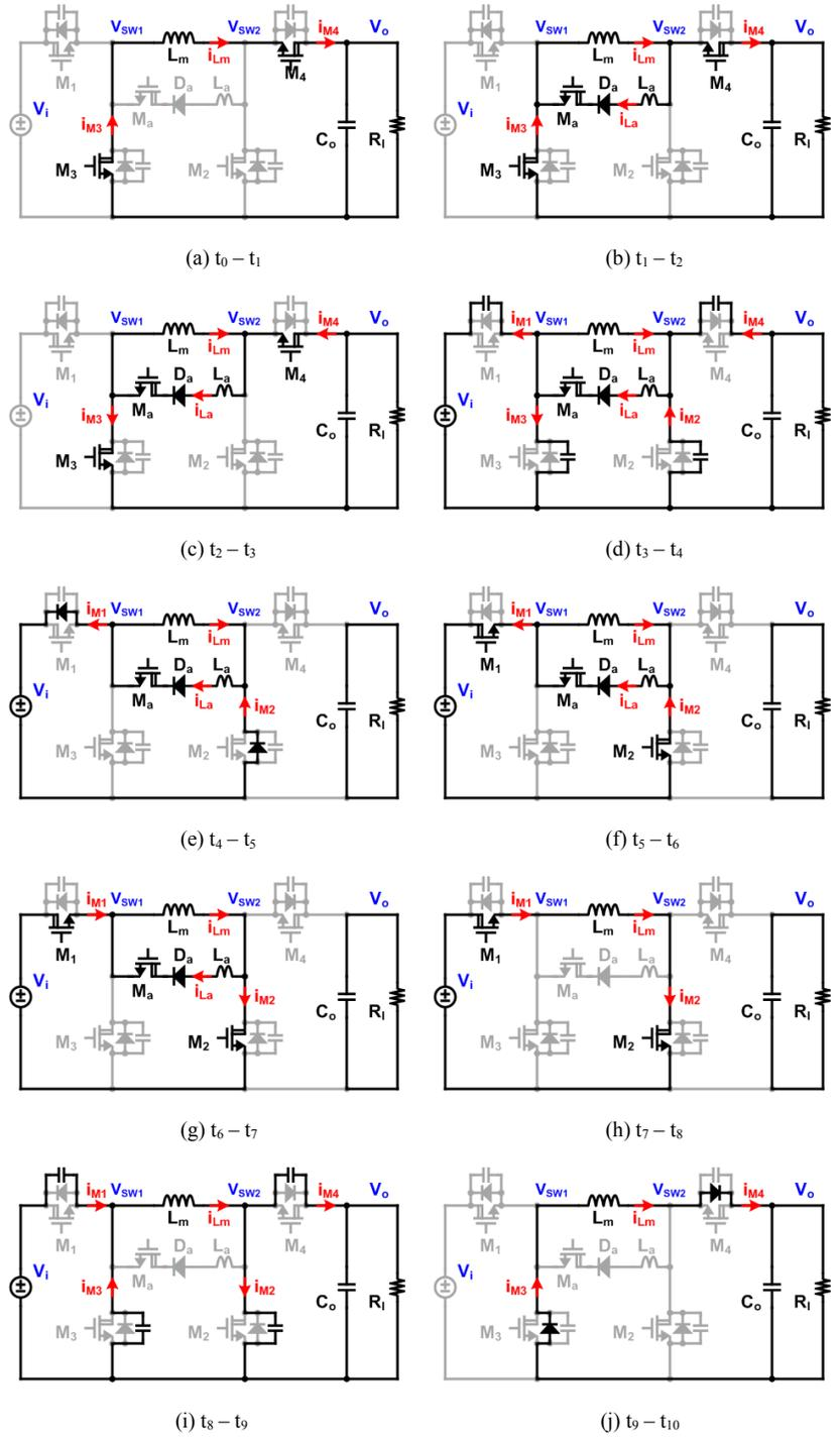
Figure 5.3. Operation states of the proposed buck-boost converter in the buck-boost mode.
