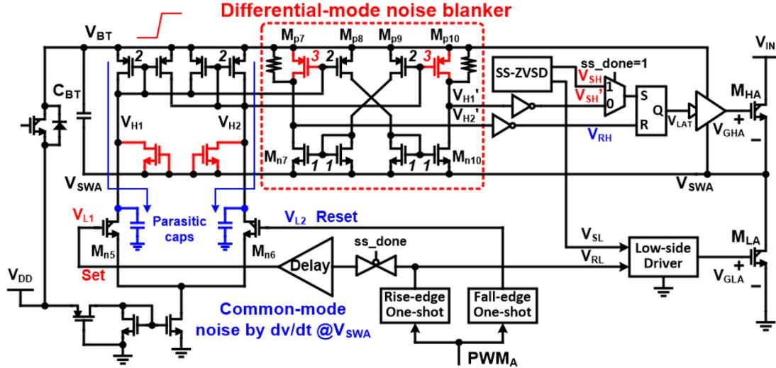
Figure 3.8. Structure of the proposed HV level shifter with the differential-mode noise blanking circuit for enhanced reliability.
