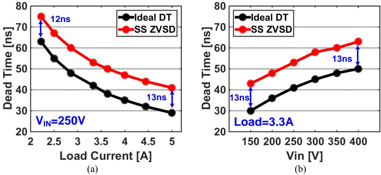
Figure 3.13. Measured dead-time under different (a) load-current and (b) input-voltage conditions.
