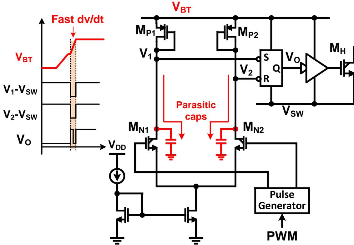
Figure 2.2. Design challenge of the HV level shifter during fast transition.
