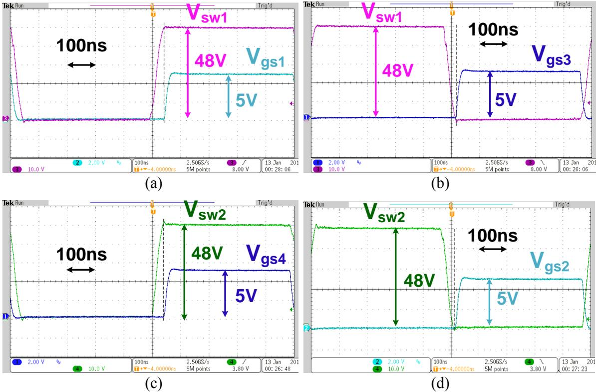
Figure 5.10. Switching transitions during the turn-on moments of (a)  $M_1$ , (b)  $M_3$ , (c)  $M_4$ , and (d)  $M_2$  of the proposed converter in the buck-boost mode at 1-MHz frequency, 48-V  $V_i$ , 48-V  $V_o$  and 0.2-A load current.
