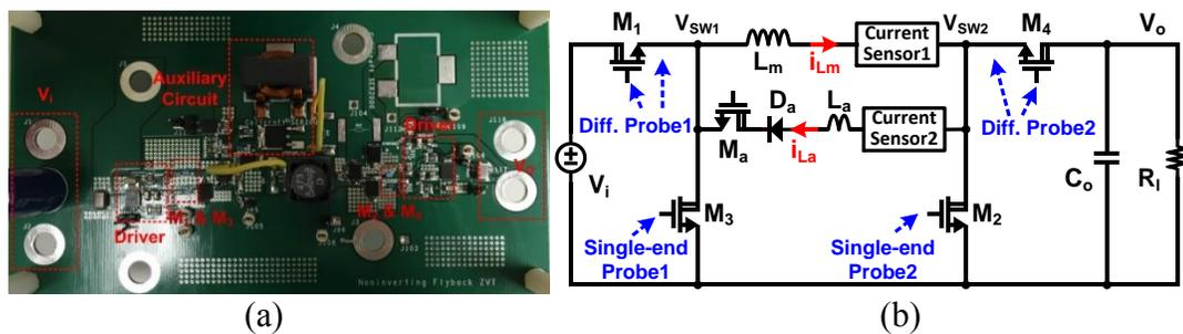
Figure 5.9. (a) Hardware prototype and (b) measurement setup of the proposed ZVT buck-boost converter.
