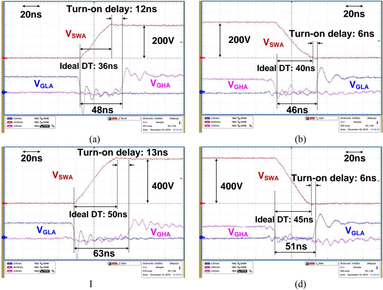
Figure 3.11. Measured  $t_{total\_delay}$  in full-ZVS operation for (a) high-side and (b) low-side power FETs at  $V_I = 200\text{ V}$ ,  $I_O = 4\text{ A}$ , and (c) high-side and (d) low-side power FETs at  $V_I = 400\text{ V}$ ,  $I_O = 4\text{ A}$ .
