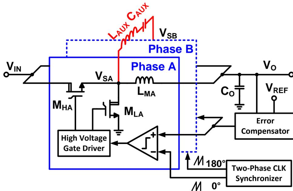
Figure 4.5. Schematic of the PS-TPZVS buck converter.
