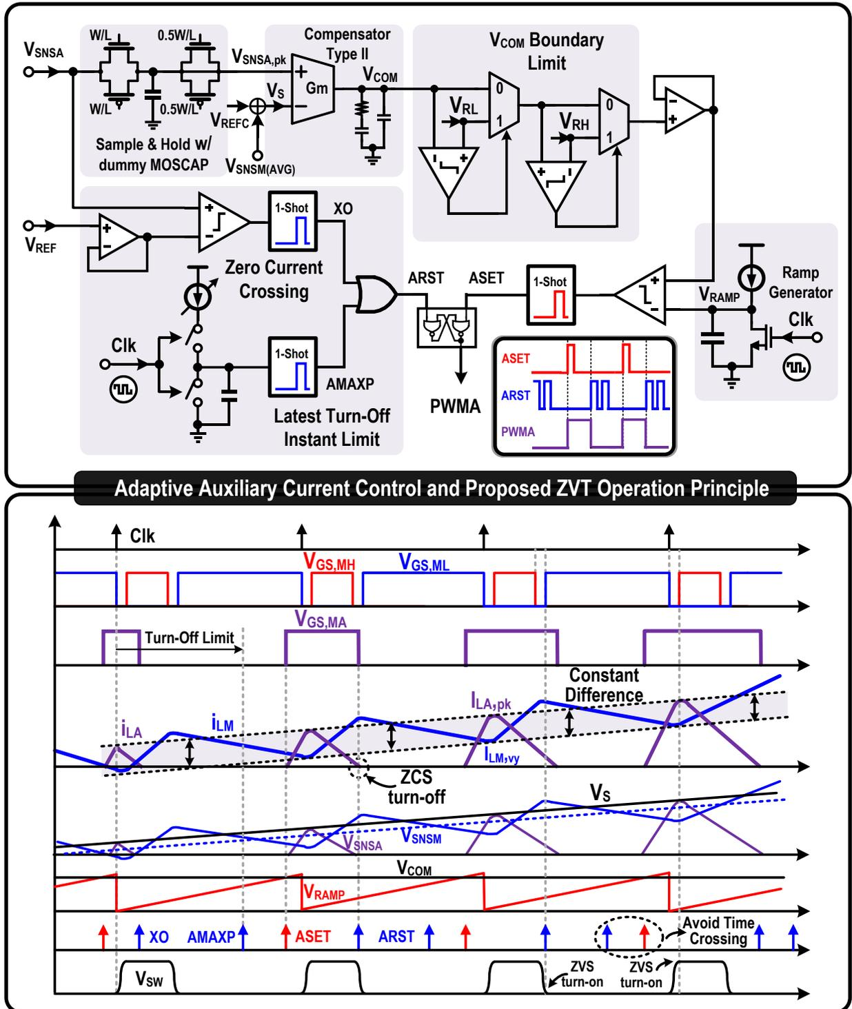
Figure 5.16. Structure and operation of the proposed adaptive auxiliary current controller.
