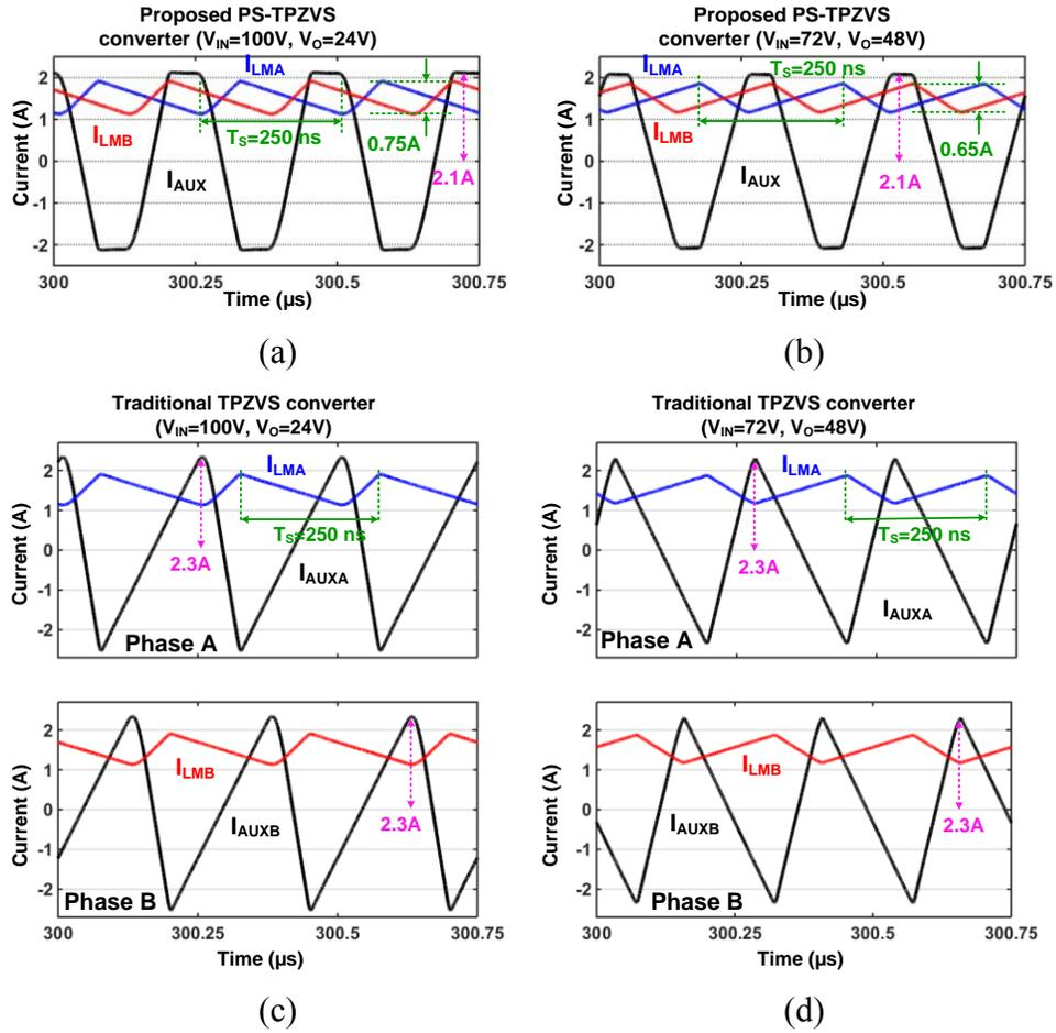
Figure 4.6. Simulated steady-state waveforms of the proposed PS-TPZVS converter under the full load of 3A: main inductor currents and auxiliary inductor current under (a)  $V_{IN} = 100\text{ V}$ ,  $V_O = 24\text{ V}$  and (b)  $V_{IN} = 72\text{ V}$ ,  $V_O = 48\text{ V}$ . The simulated main inductor current and the auxiliary inductor current of the traditional two-phase ZVS converter are provided in (c) and (d) with the same conditions of (a) and (b), respectively.
