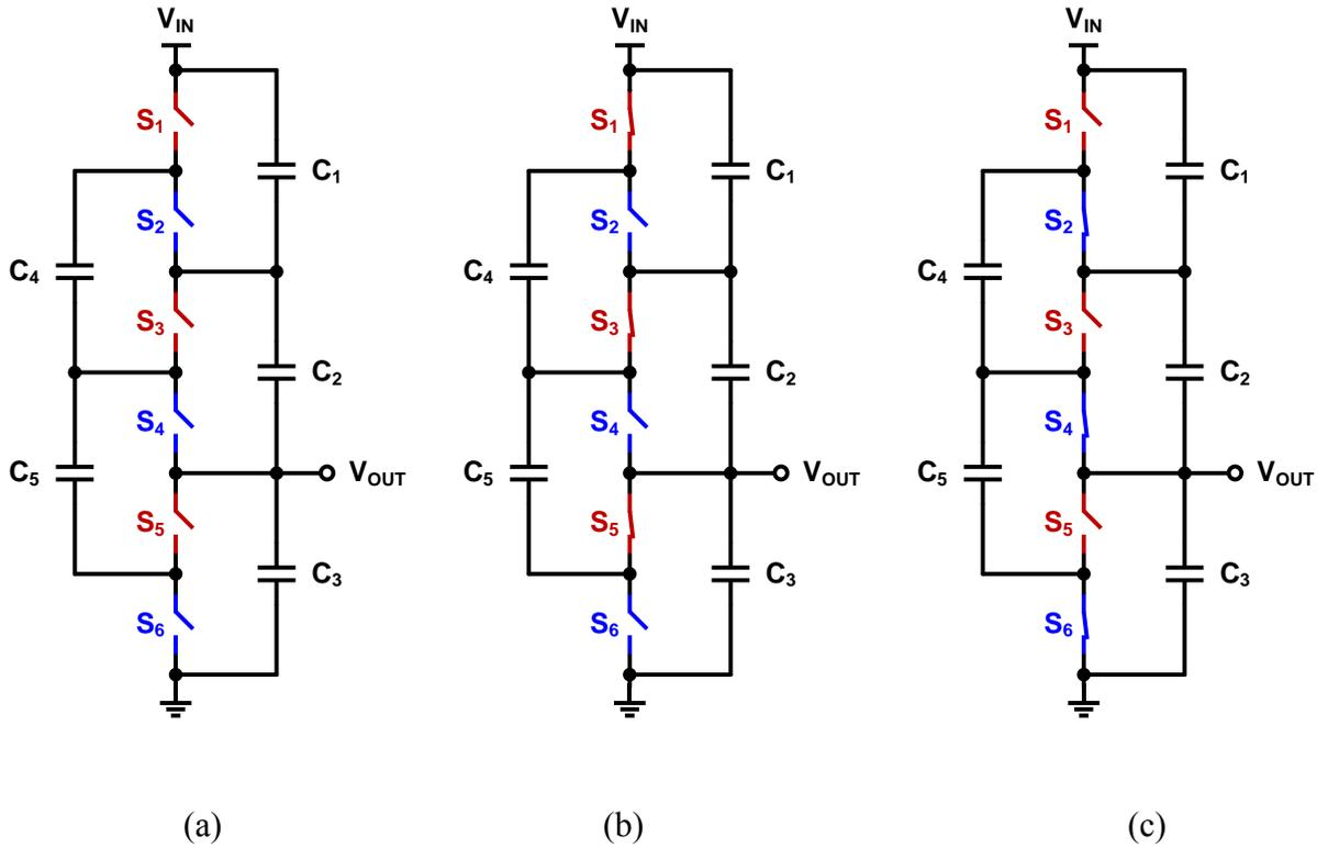
Figure 1.2. (a) A switched capacitor converter in 3-to-1 ladder topology, including networks in (b) phase 1 and (c) phase 2.
