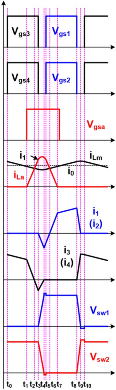
Figure 5.2. Key waveforms in the buck-boost mode.
