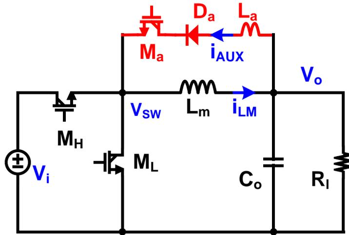
Figure 2.6. Schematic of ZVT buck converter.
