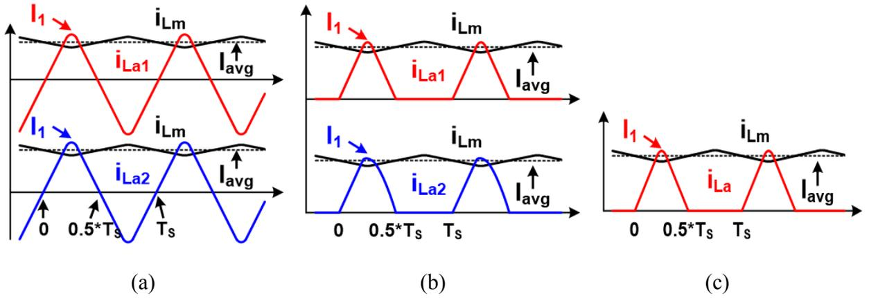
Figure 5.7. Main and auxiliary inductor current waveforms of the non-inverting buck-boost converters using (a) the QSW-ZVS, (b) the traditional ZVT, and (c) the proposed ZVT.
