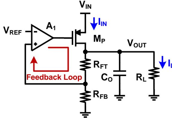
Figure 1.1. Schematic of a low-dropout regulator.
