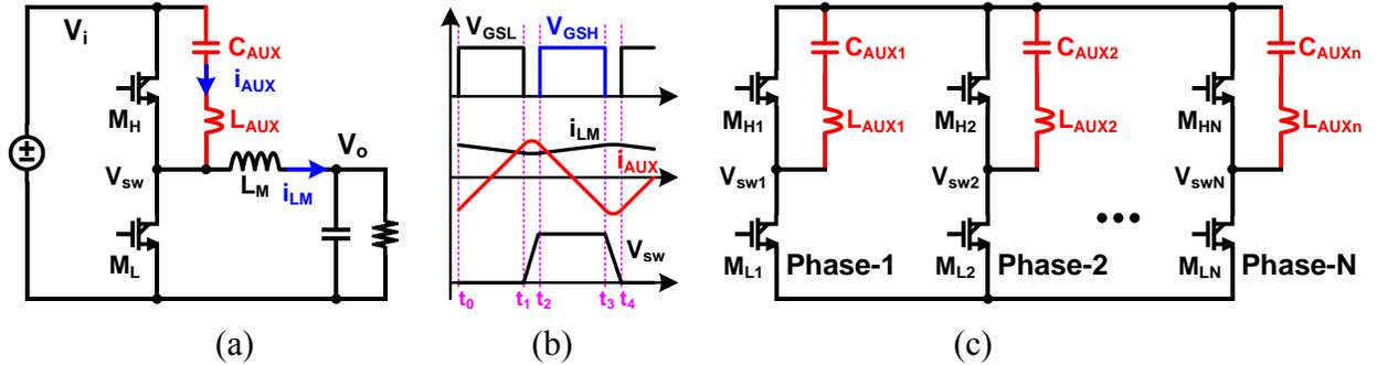
Figure 2.3. (a) schematic of QSW-ZVS buck converter; (b) waveforms of QSW-ZVS buck converter; (c) N-phase QSW-ZVS topology.
