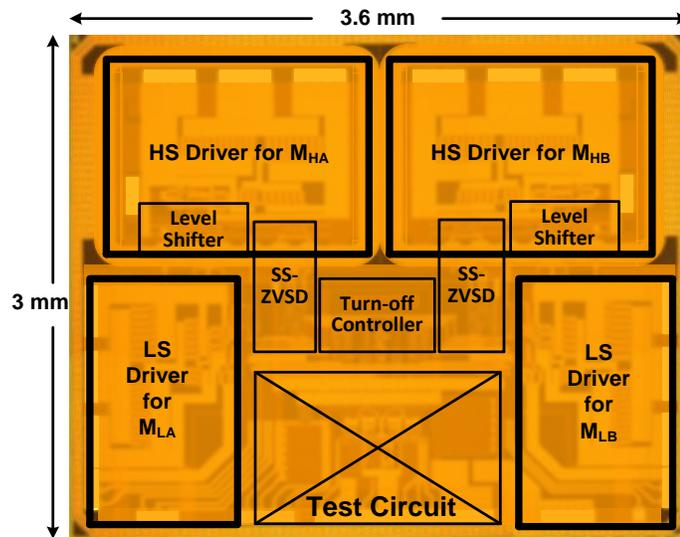
Figure 3.10. Micrograph of the proposed ZVS gate driver for the full-bridge converter using eGaN power FETs.
