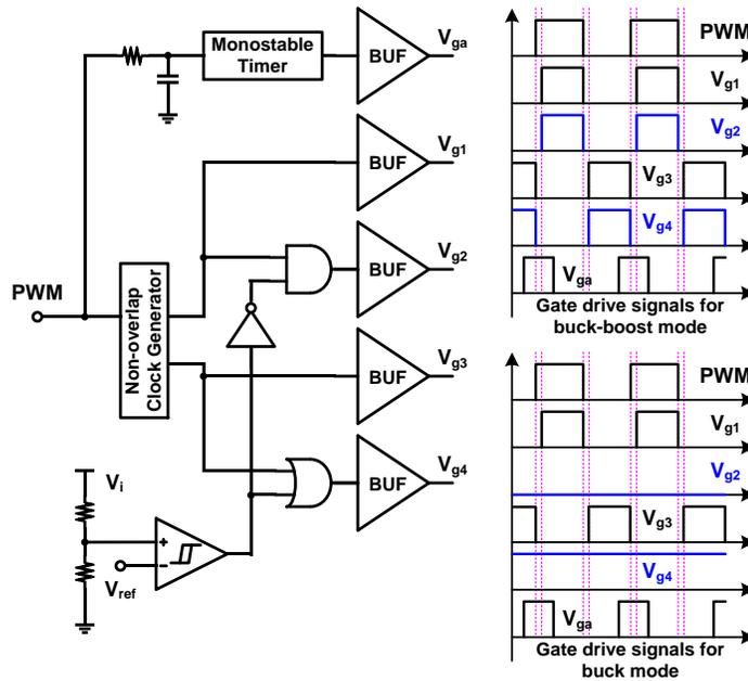
Figure 5.8. Gate driver structure of the proposed non-inverting buck-boost converter.
