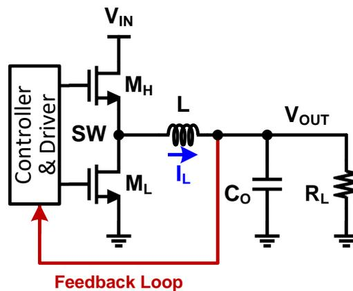
Figure 1.3. Schematic of a buck converter.
