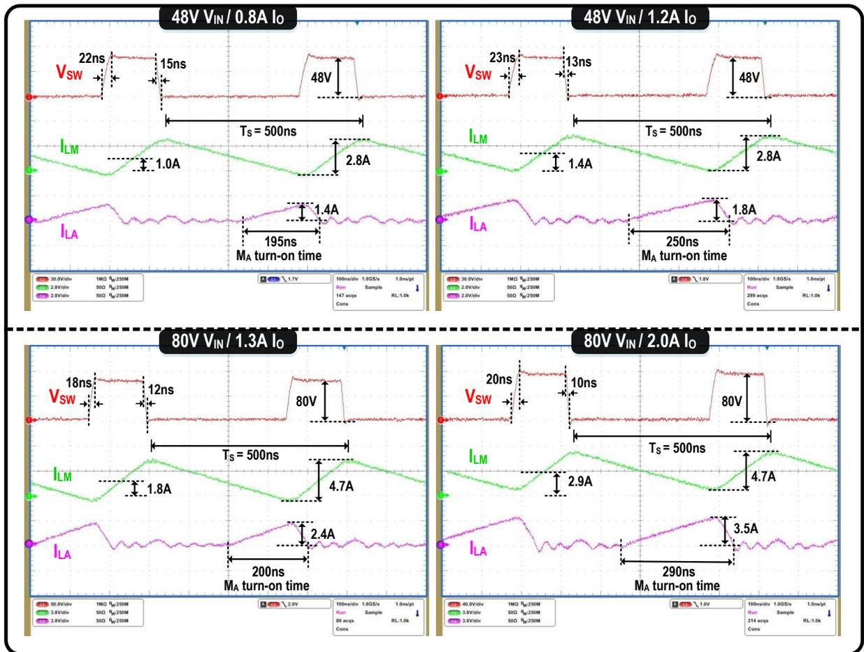
Figure 5.18. Measured steady-state waveforms under different  $V_{IN}$  and  $I_O$  conditions in the AZVT mode.
