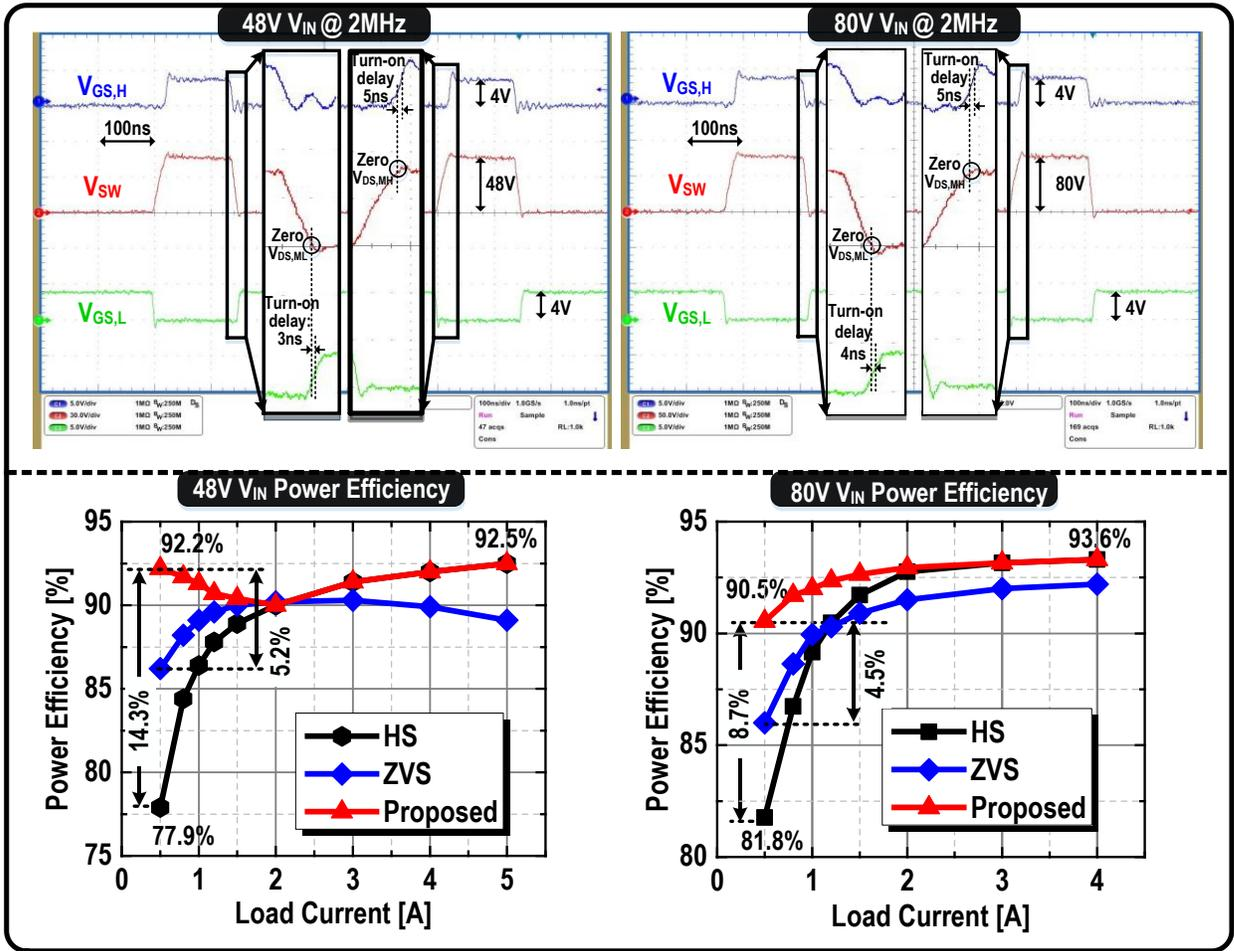
Figure 5.19. Measured ZVS operation and turn-on delays of high-side and low-side GaN FETs, and measured converter power efficiencies at 2MHz  $f_{sw}$  under different  $V_{IN}$  and  $I_O$  conditions.
