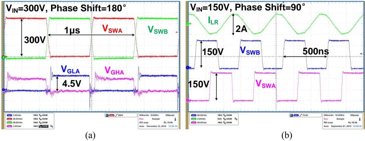
Figure 3.14. Measured converter steady-state waveforms at (a)  $V_I = 300\text{ V}$ ,  $I_O = 5\text{ A}$ , phase shift =  $180^\circ$  and (b)  $V_I = 150\text{ V}$ ,  $I_O = 5\text{ A}$ , phase shift =  $90^\circ$ .
