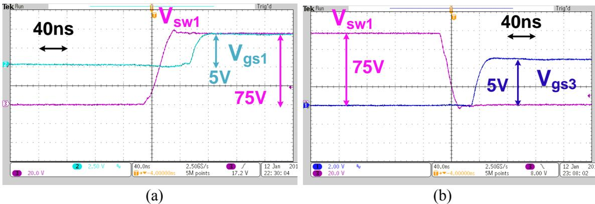
Figure 5.11. Switching transitions during the turn-on moments of (a)  $M_1$  and (b)  $M_3$  of the proposed converter in the buck mode at 1-MHz frequency, 75-V  $V_i$ , 48-V  $V_o$  and 1.2-A load current.
