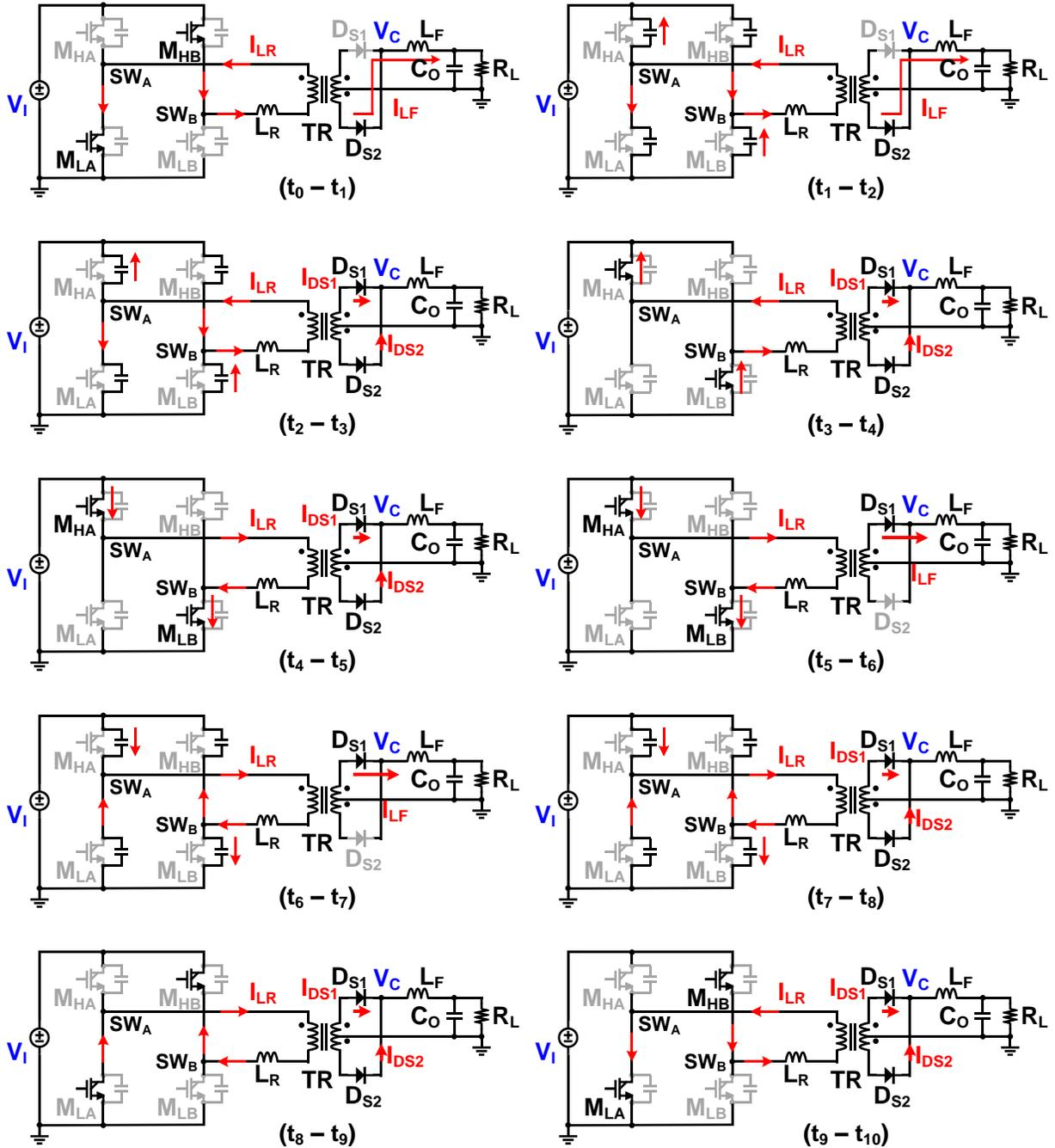
Figure 3.3. Converter states in different time subintervals of a period for full-ZVS operation.
