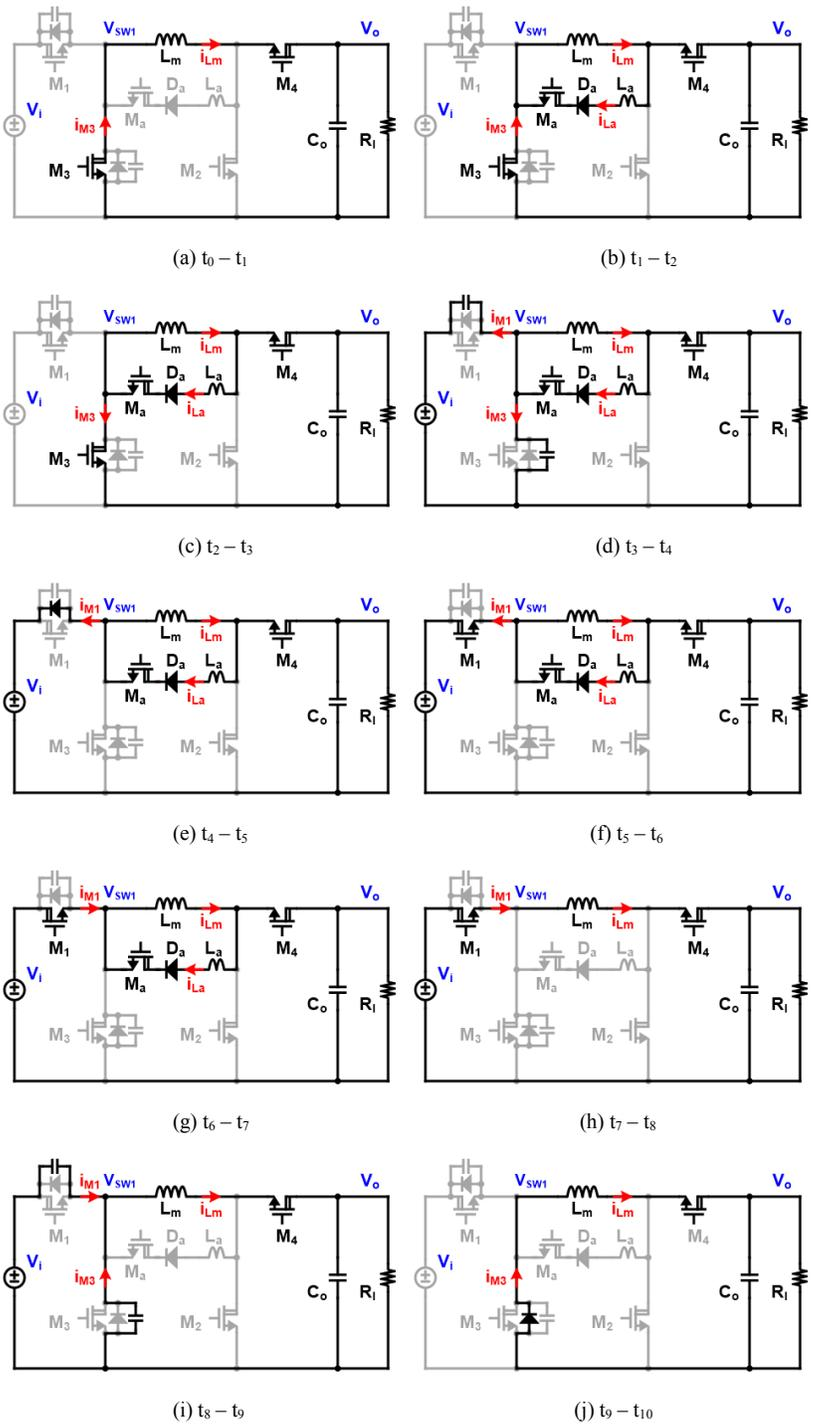
Figure 5.5. Operation states of the proposed buck-boost converter in the buck mode.
