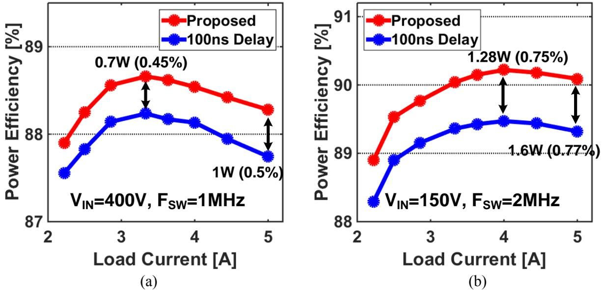
Figure 3.15. Measured power efficiency under (a)  $V_I = 400\text{ V}$  and  $F_{SW} = 1\text{ MHz}$  and (b)  $V_I = 150\text{ V}$  and  $F_{SW} = 2\text{ MHz}$ .
