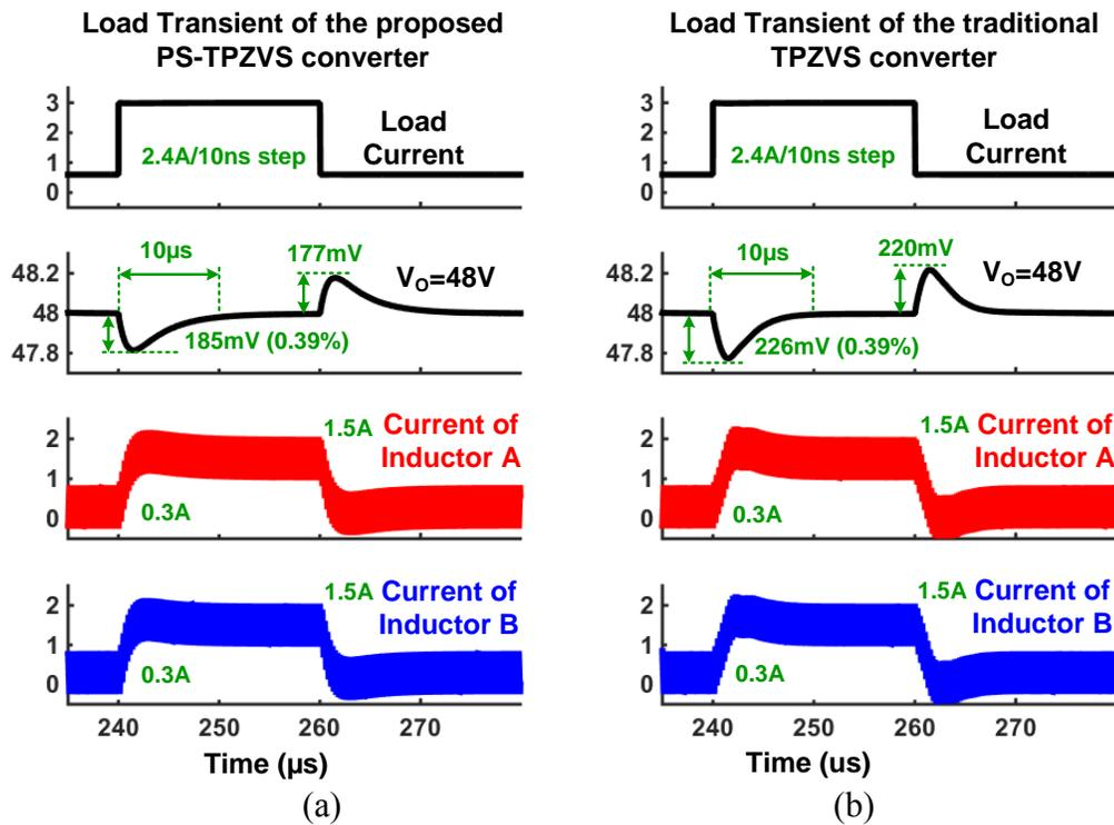
Figure 4.9. Simulated transient response of the proposed converter with a load step between 0.6 A and 3 A (load current slew rate: 2.4 A/ 10 ns) for (a) the proposed PS-TPZVS buck converter at 4 MHz and (b) traditional two-phase ZVS buck converter at 4 MHz.
