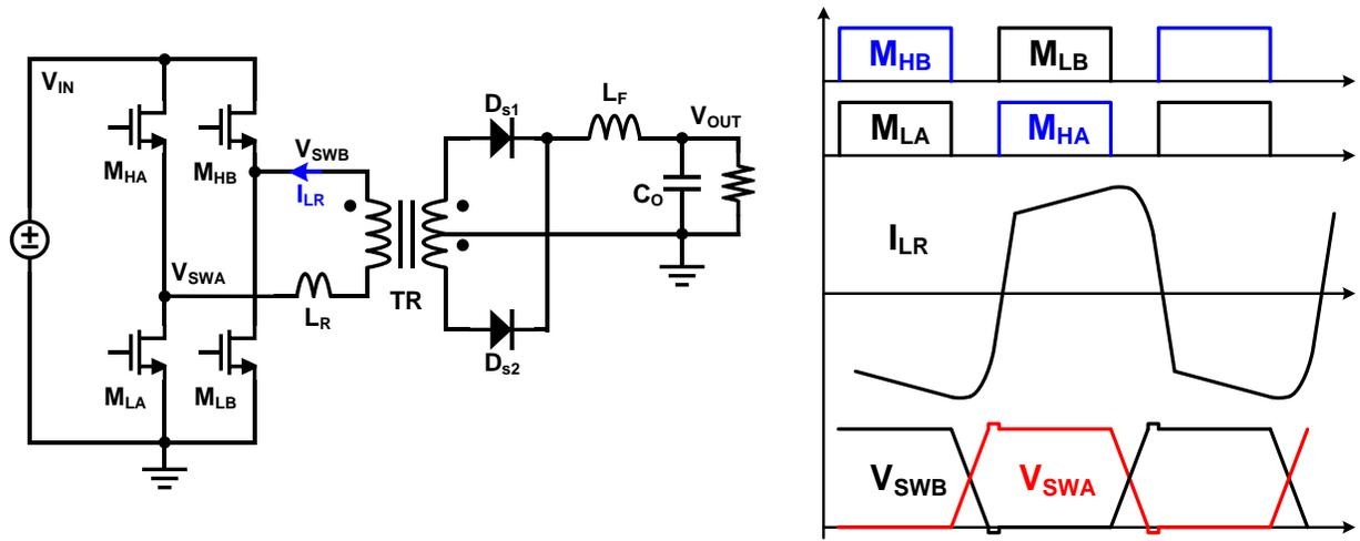
Figure 1.7. Schematic and waveforms of an isolated full-bridge ZVS converter.
