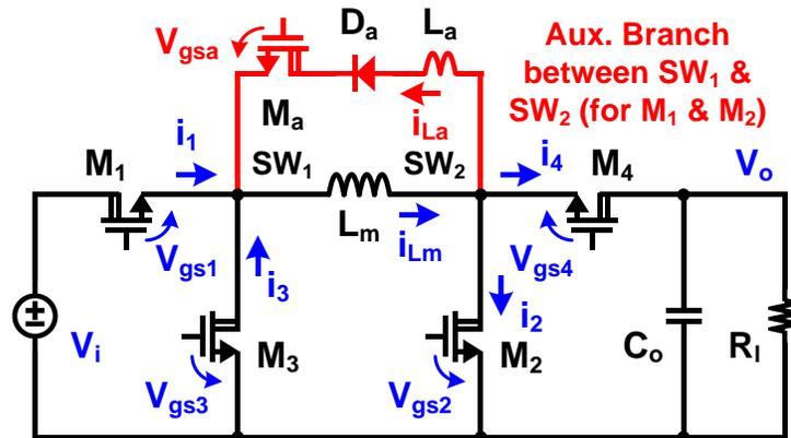
Figure 5.1. Schematic of the proposed ZVT synchronous non-inverting buck-boost converter with the shared auxiliary circuit.
