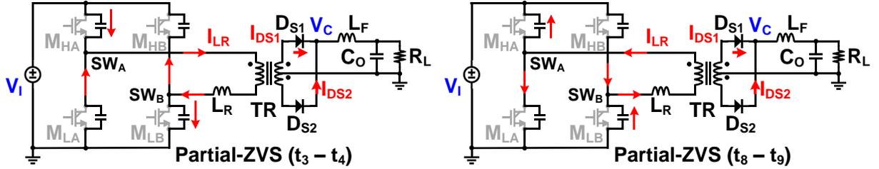
Figure 3.4. Partial-ZVS operation states that are different from those in the full-ZVS operation.
