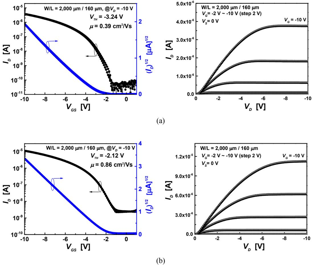
Figure 3. Current-voltage transfer (left) and output (right) characteristics of TIPS-pentacene/PTAA transistors on (a) SMP and (b) glass substrates
