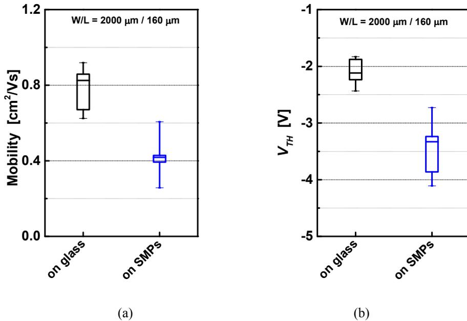
Figure 4. Comparison of (a) mobility and (b) threshold voltages of OFETs on SMP and glass substrates.
