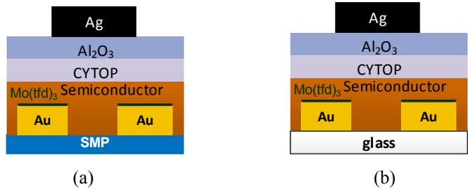
Figure 2. Vertical structure of fabricated OFETs on (a) SMP and (b) glass substrates.
