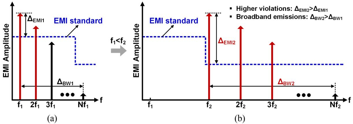
Figure 1.4. EMI spectra comparison under (a) low switching frequency and (b) high switching frequency in switching power circuits.
