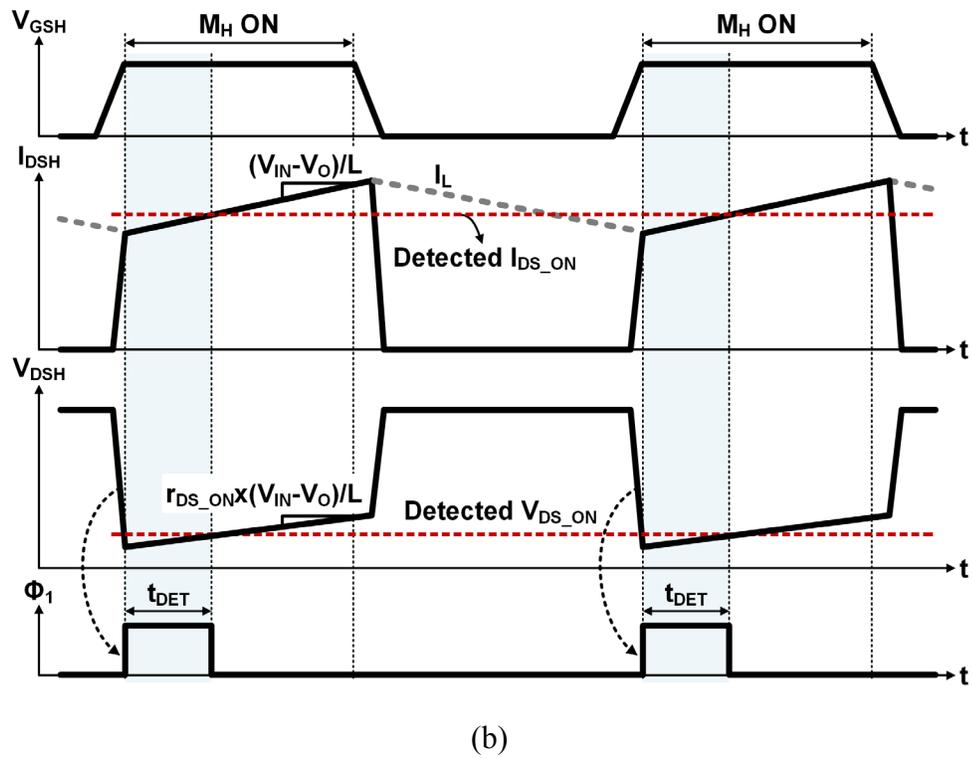
Figure 2.4. Proposed  $r_{DS\_ON}$ -based online condition monitor. (a) Circuit block diagram and (b) timing diagram.
