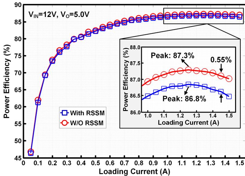
Figure 4.20. Measured efficiency.
