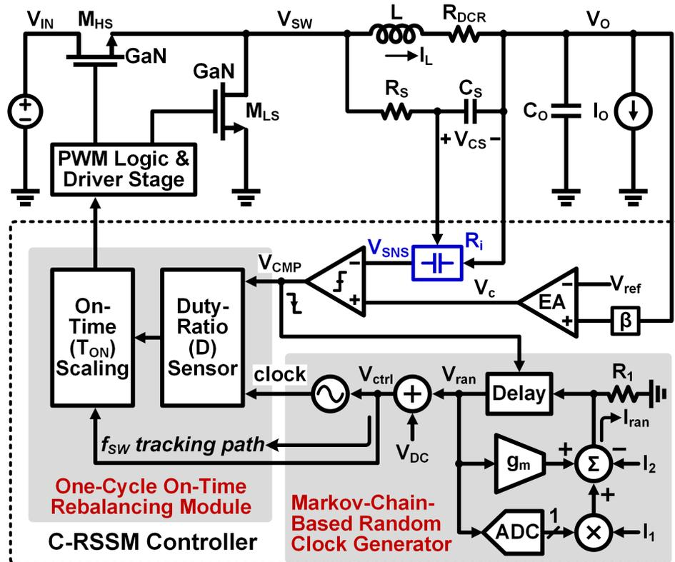
Figure 4.11. Block diagram of the GaN power system with C-RSSM control.
