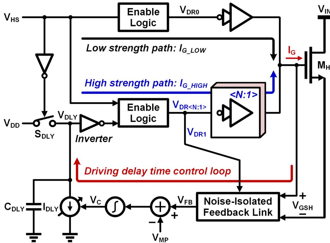
Figure 3.6. Block diagram of adaptive strength gate driving scheme.
