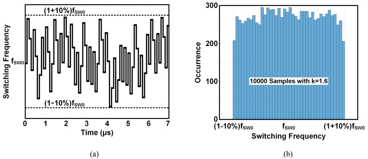
Figure 4.8. Simulations of the random clock generator based on Markov chain: (a) switching frequency dithering in time domain, and (b) switching frequency distribution.
