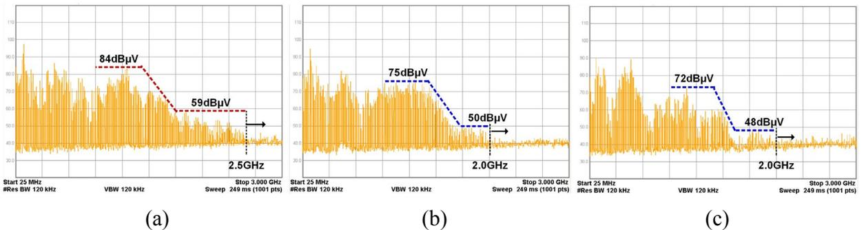
Figure 3.13. Measured EMI spectra in Band C/D (> 30MHz) under different operation modes: (a) high di/dt and high dv/dt, (b) proposed work with low di/dt and high dv/dt, and (c) low di/dt and low dv/dt.
