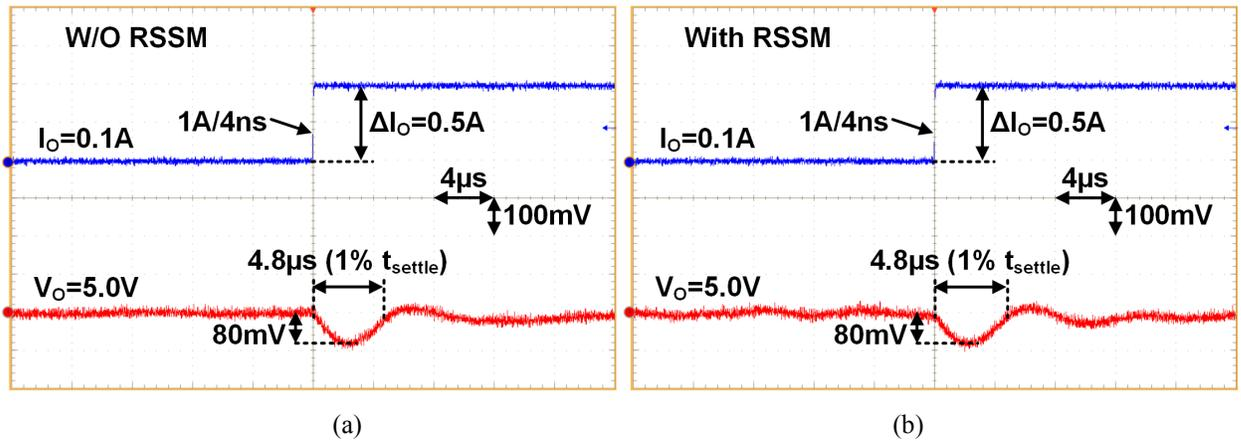
Figure 4.19. Measured dynamic performance of the power converter with load current rising: (a) without, and (b) with the proposed Markov C-RSSM.
