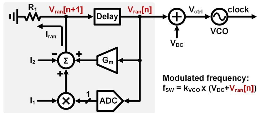
Figure 4.5. Block diagram of the proposed random clock generator based on Markov chain with fundamental analog modules.
