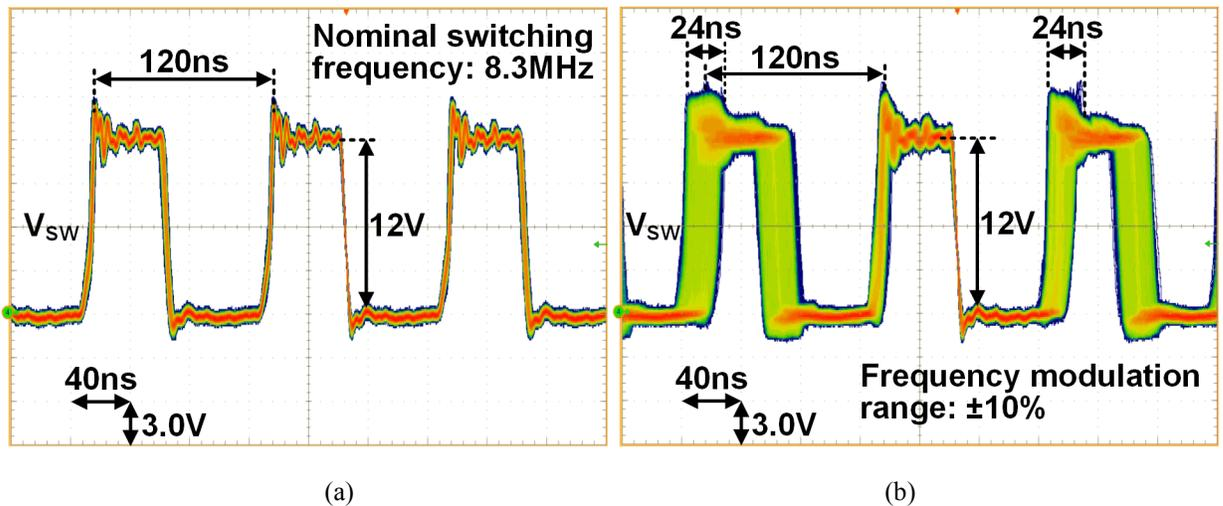
Figure 4.15. Measured waveforms at the switching node  $V_{sw}$ : (a) without, and (b) with the Markov C-RSSM scheme.
