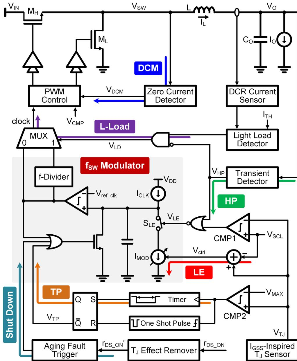
Figure 2.8. Circuit schematic of proactive temperature frequency scaling scheme.
