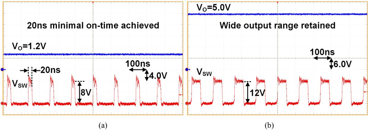
Figure 4.18. Measured switching node  $V_{SW}$  with reference to variable output voltages: (a)  $V_O=1.2V$ , and (b)  $V_O=5.0V$ .
