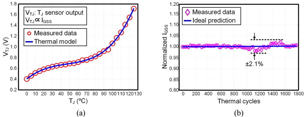
Figure 2.13. Measured results on the gate leakage  $I_{GSS}$ -inspired  $T_J$  sensing: (a) on-chip sensed voltage  $V_{TJ}$  versus  $T_J$ , and (b)  $I_{GSS}$  versus thermal cycles.
