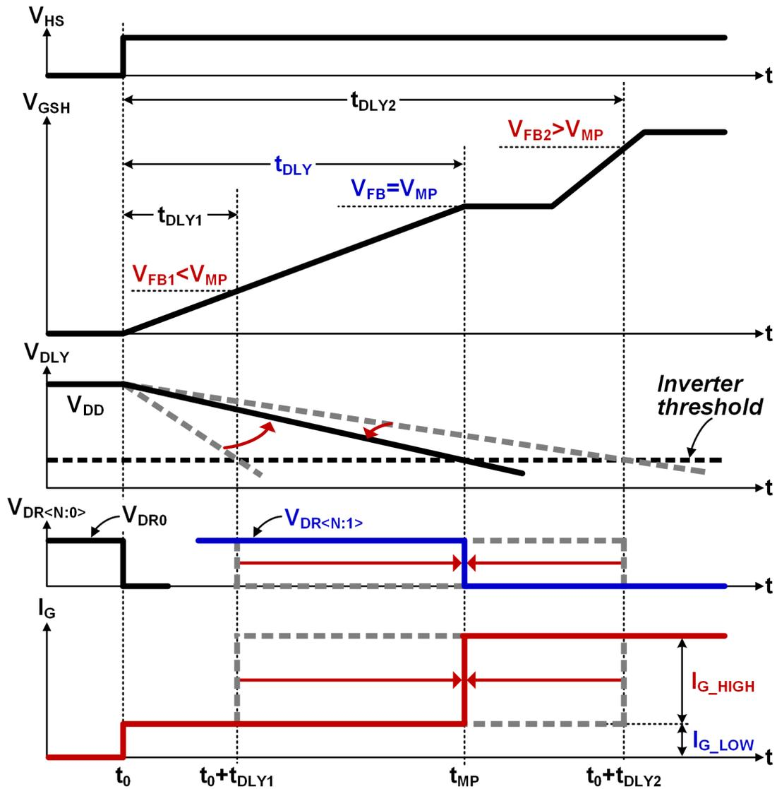
Figure 3.7. Operation principle of adaptive strength gate driving scheme.
