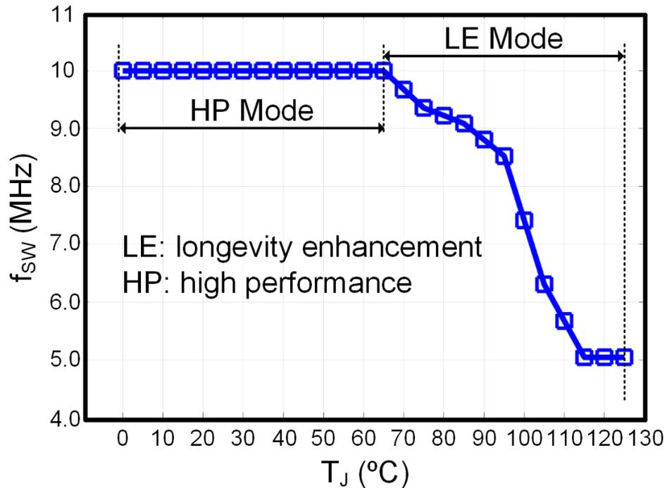
Figure 2.15. Measured results on the temperature frequency scaling scheme.
