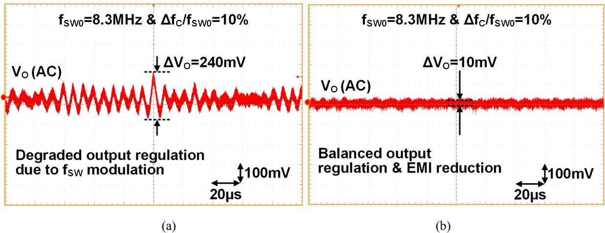
Figure 4.17. Measured jittering effect at the output node when applying RSSM with (a) classical PWM scheme, and (b) designed one-cycle on-time rebalancing methodology.
