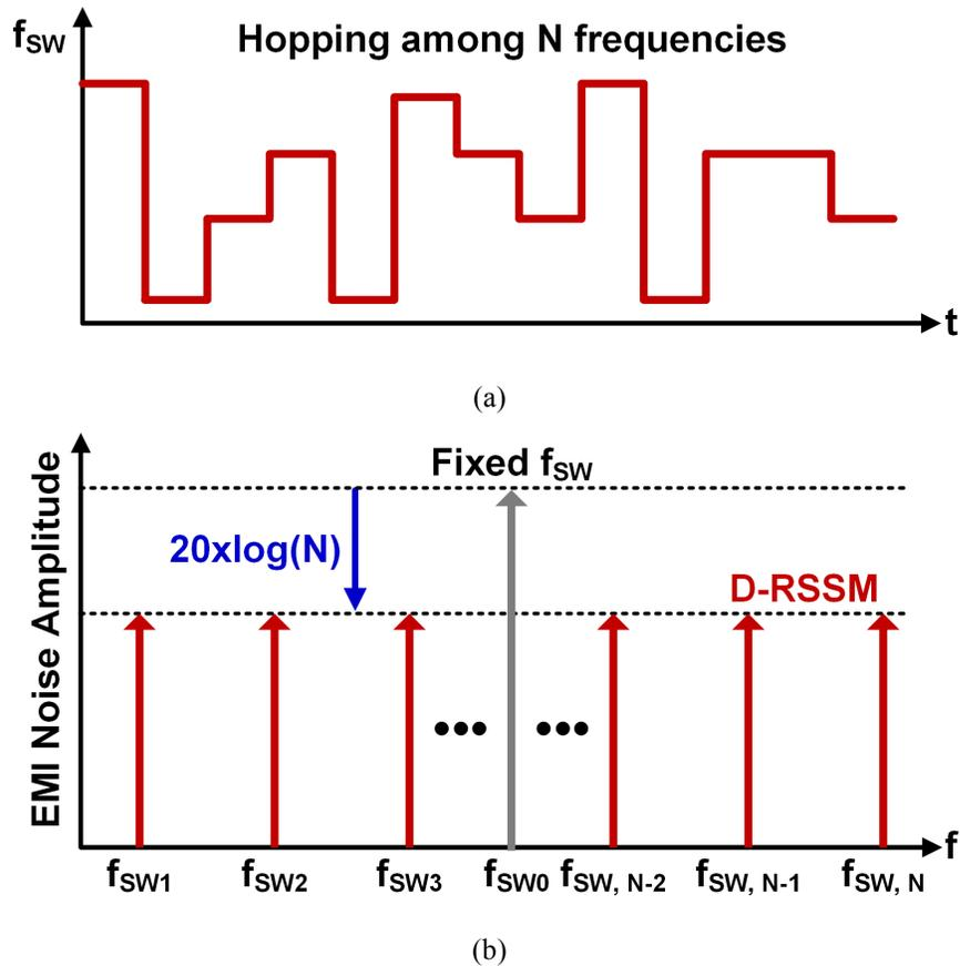
Figure 4.2. Conventional discrete RSSM (D-RSSM) technique: (a) frequency hopping within finite values, and (b) EMI spectral redistribution.
