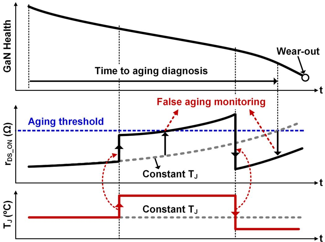
Figure 2.2. False aging monitoring induced by temperature fluctuations.
