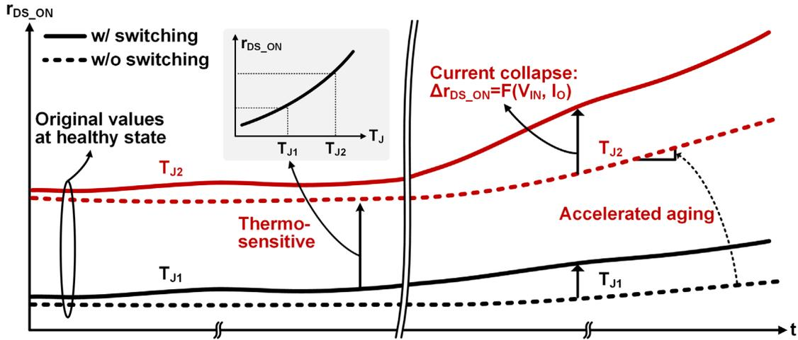
Figure 1.2. Dependence of dynamic on-resistance  $r_{DS\_ON}$  on switching conditions and junction temperature  $T_J$ .
