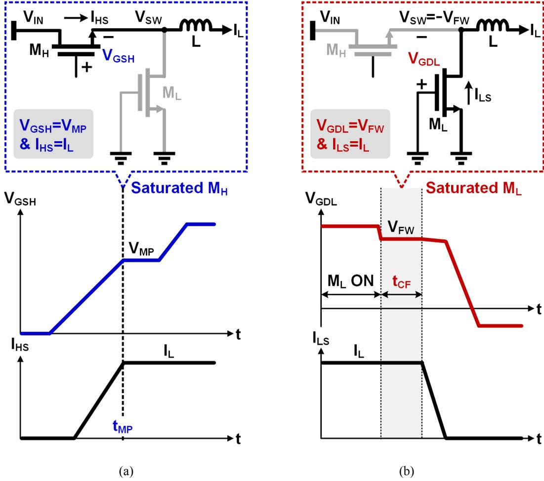
Figure 3.5. Basic principle of emulated Miller Plateau tracking scheme: (a)  $M_H$  switching behavior at Miller Plateau starting point  $t_{MP}$ , and (b)  $M_L$  switching behavior during current freewheeling period  $t_{CF}$ .
