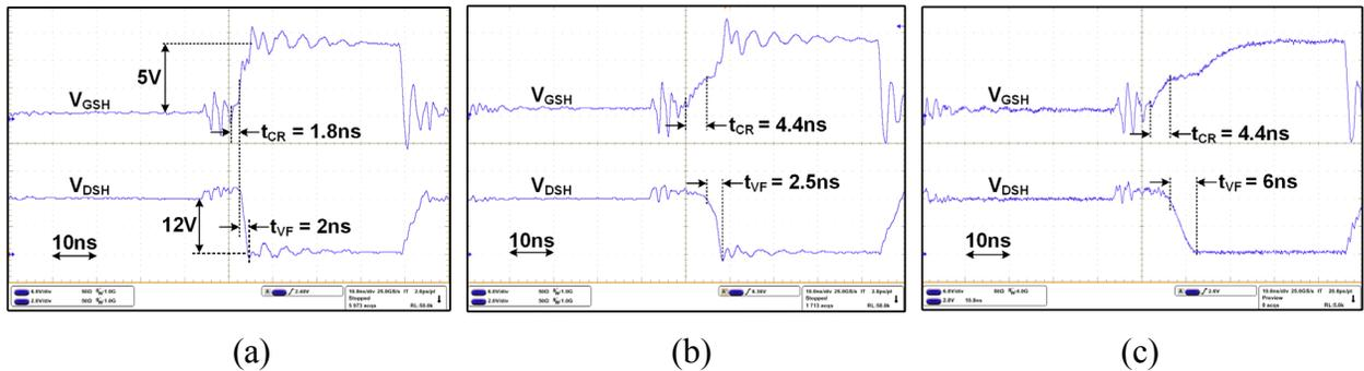
Figure 3.15. Measured waveforms of high side gate-source voltage  $V_{GS}$  and drain-source voltage  $V_{DS}$  under different operation modes: (a) high  $di/dt$  and high  $dv/dt$ , (b) proposed work with low  $di/dt$  and high  $dv/dt$ , and (c) low  $di/dt$  and low  $dv/dt$ .
