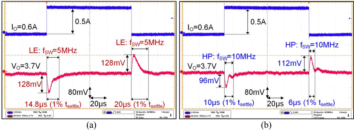
Figure 2.16. Comparison of load transient response under (a) longevity-enhancement (LE) mode and (b) high-performance (HP) mode.
