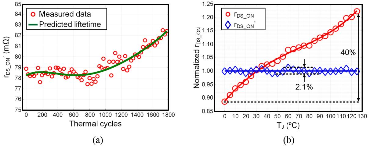
Figure 2.12. Measured results on aging precursor  $r_{DS\_ON}$ : (a) thermal stress test and (b) temperature dependence calibration.
