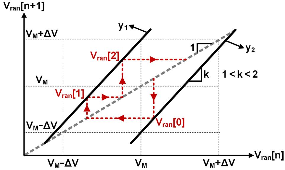
Figure 4.4. Chaotic piecewise-linear one-dimensional (PL1D) map for designing Markov-chain-based random voltage source.
