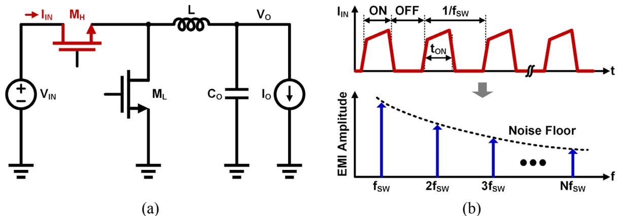
Figure 1.3. Illustration of EMI issue: (a) DC-DC buck converter and (b) conducted EMI noise due to switching actions.
