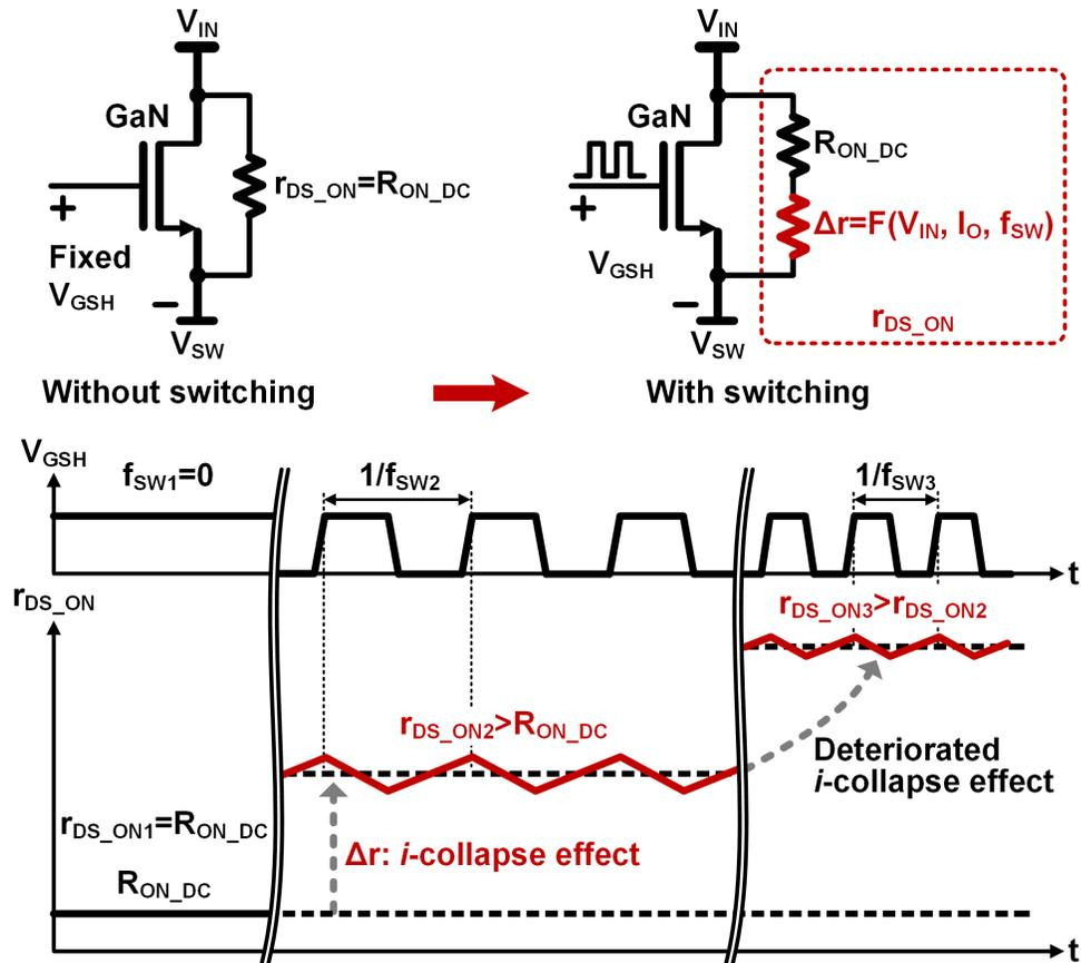
Figure 2.3. Dependence of dynamic on-resistance on specific switching conditions.
