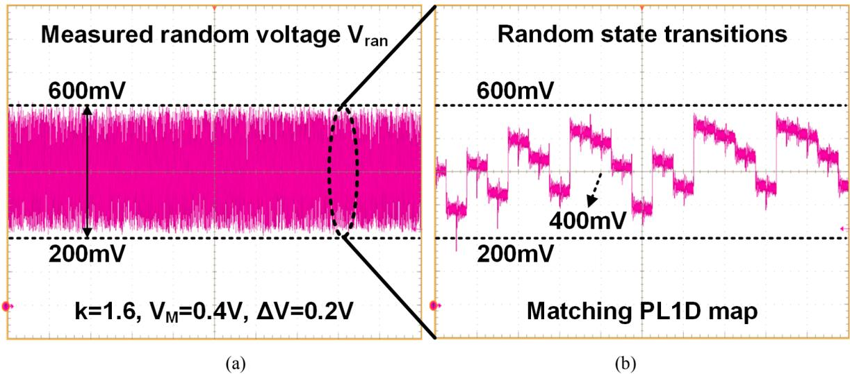
Figure 4.14. Measured random voltage  $V_{ran}$  in the random clock generator based on Markov chain: (a) state space boundary, and (b) state transitions.
