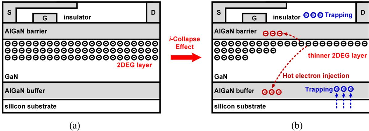
Figure 1.1. Device-level aging mechanism in GaN power switches: (a) healthy state and (b) *i*-collapse effect due to hot electron injection and charge trapping.
