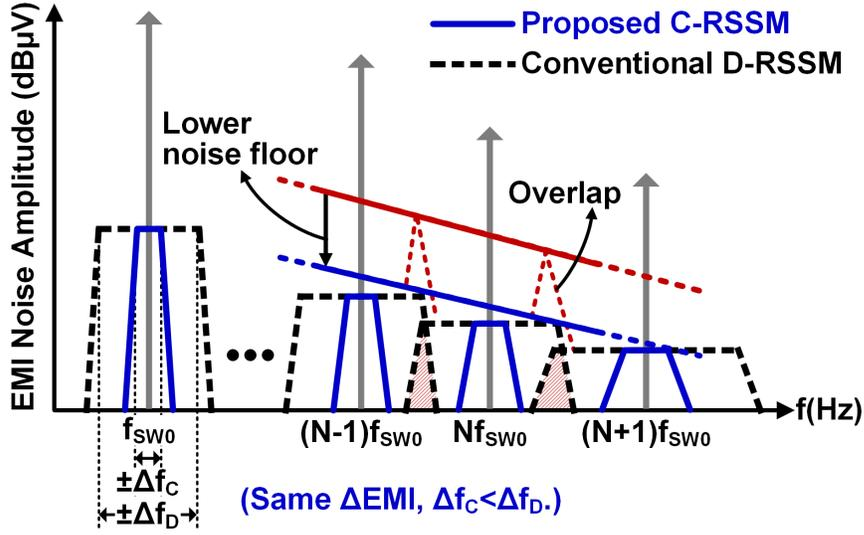
Figure 4.6. Illustration of the proposed Markov C-RSSM compared to D-RSSM.
