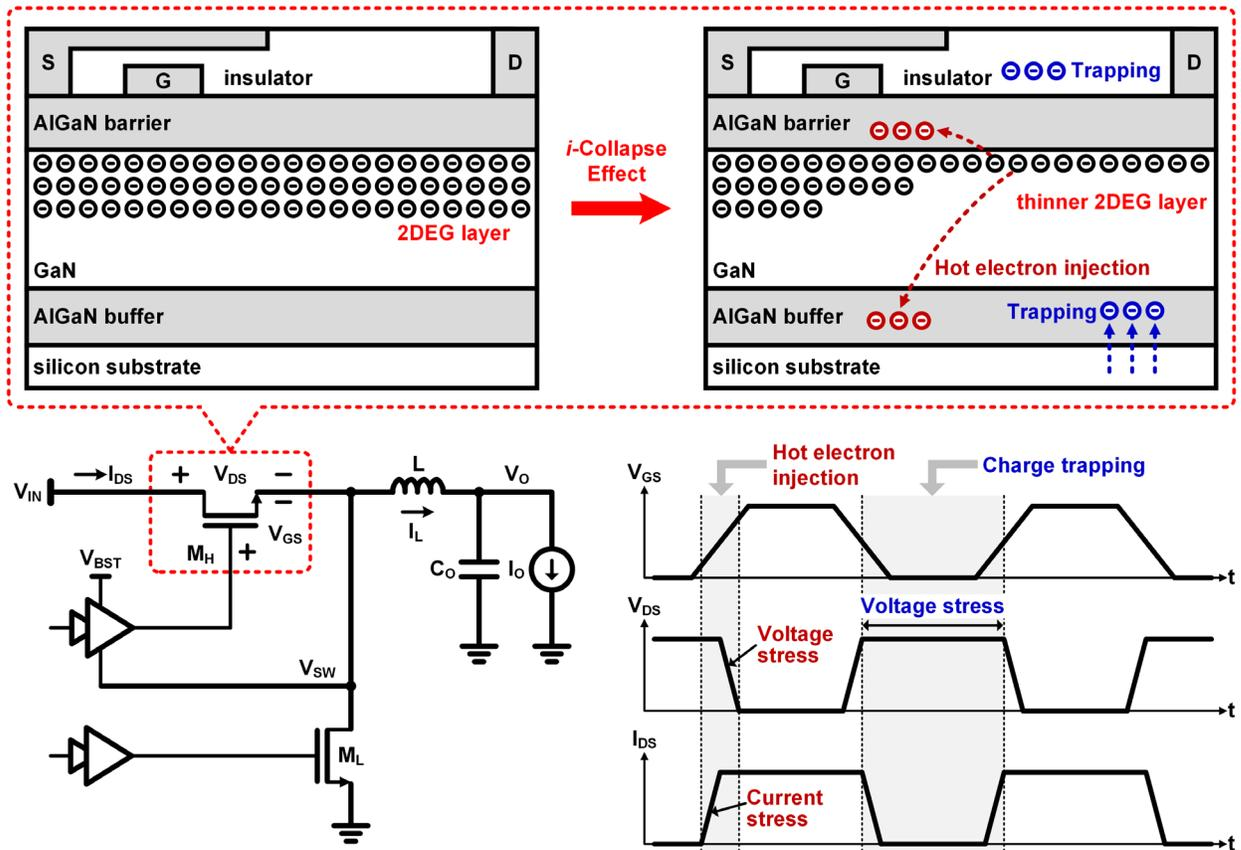
Figure 2.1. Device- and circuit-level *i*-collapse aging mechanisms in GaN power switches.
