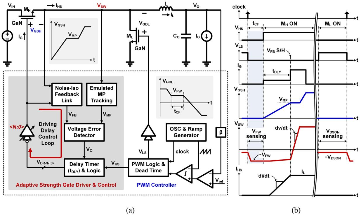
Figure 3.3. (a) System architecture of the proposed GaN buck converter, and (b) operation waveforms in steady state.
