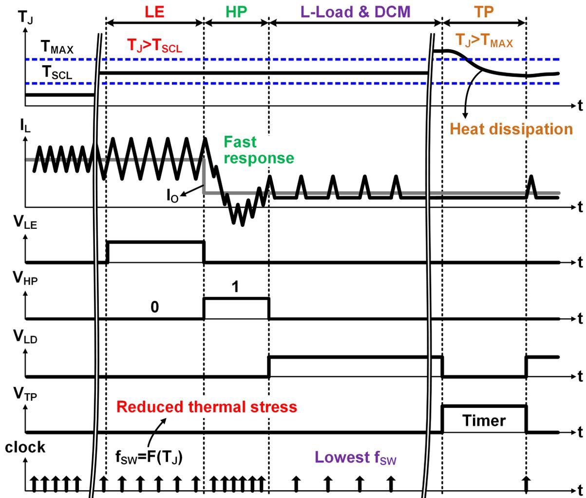
Figure 2.9. Operation principle of proactive temperature frequency scaling scheme.
