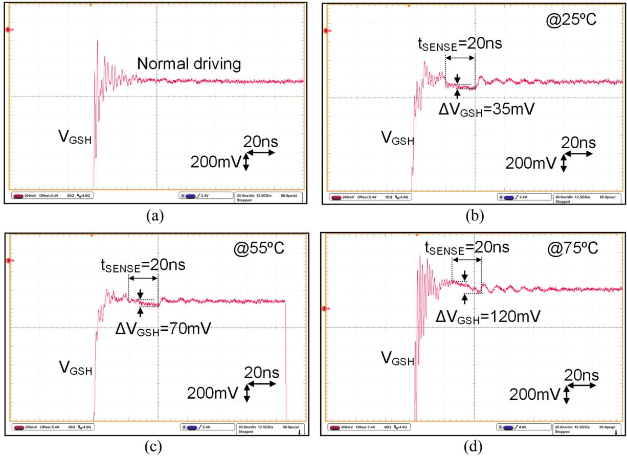
Figure 2.14. Measured GaN switch gate voltage waveforms with (a) normal driving, and  $T_J$  sensing at different temperatures of (b) 25°C, (c) 55°C and (d) 75°C.
