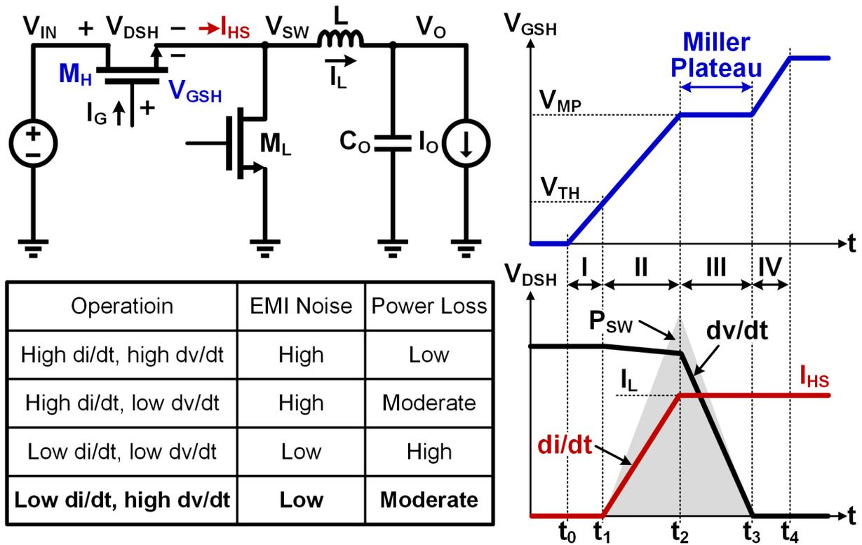
Figure 3.1. Switching V-I characteristics of the high-side switch  $M_H$  in a buck power converter demonstrating design trade-off between EMI and power loss.
