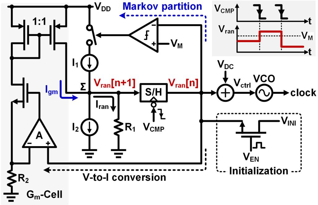
Figure 4.7. Circuit design of the proposed random clock generator based on Markov chain.
