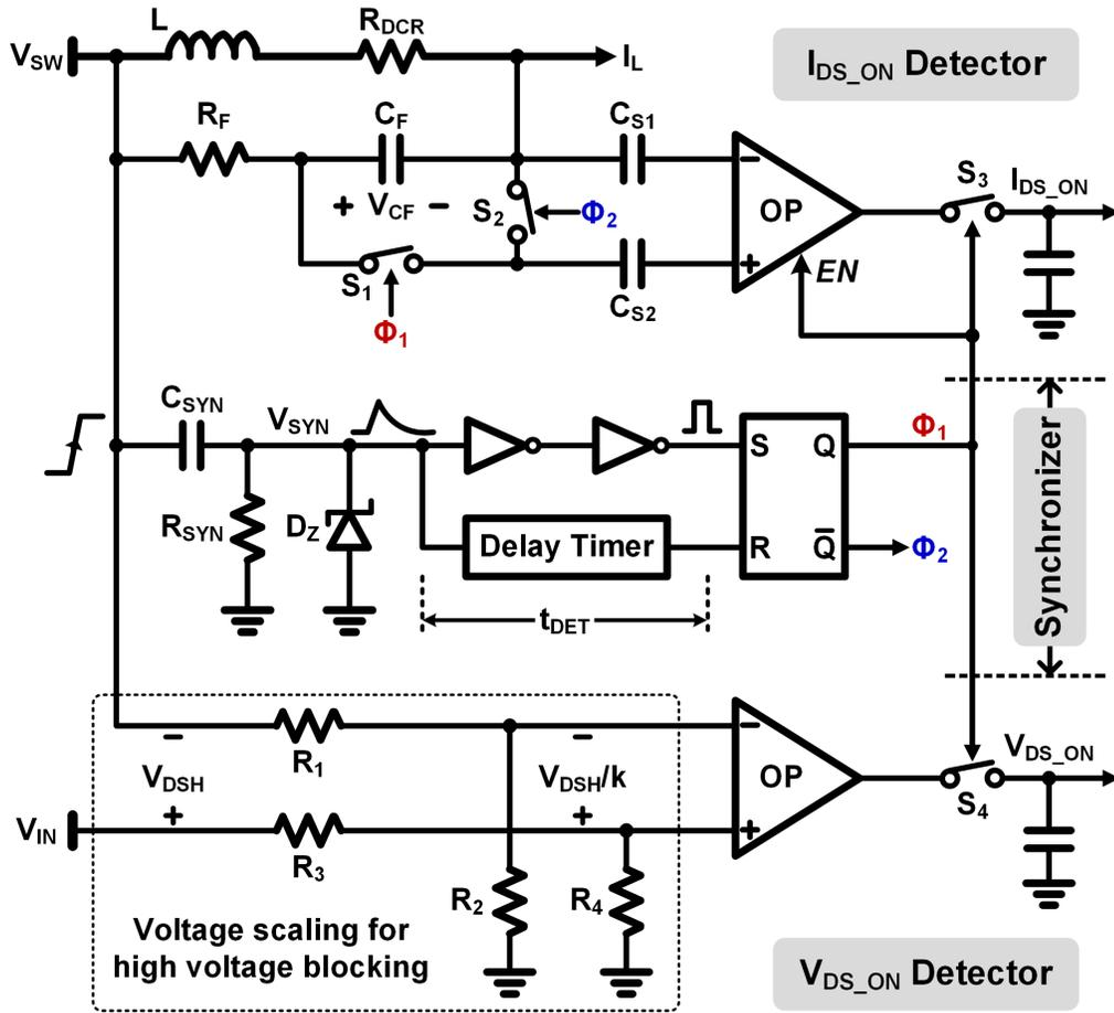
Figure 2.5. Schematic of dynamic on-resistance  $r_{DS\_ON}$  sensor.
