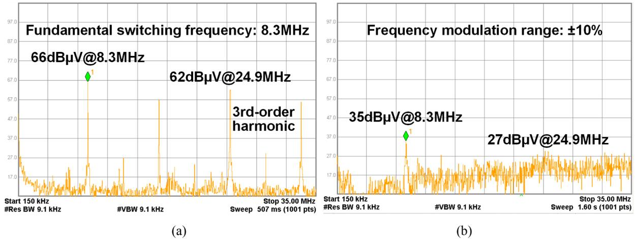
Figure 4.16. Measured conducted EMI in the frequency range below 30MHz: (a) without, and (b) with the Markov C-RSSM scheme.
