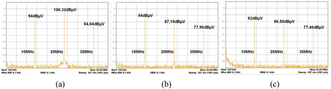
Figure 3.12. Measured EMI spectra in Band B (< 30MHz) under different operation modes: (a) high di/dt and high dv/dt, (b) proposed work with low di/dt and high dv/dt, and (c) low di/dt and low dv/dt.
