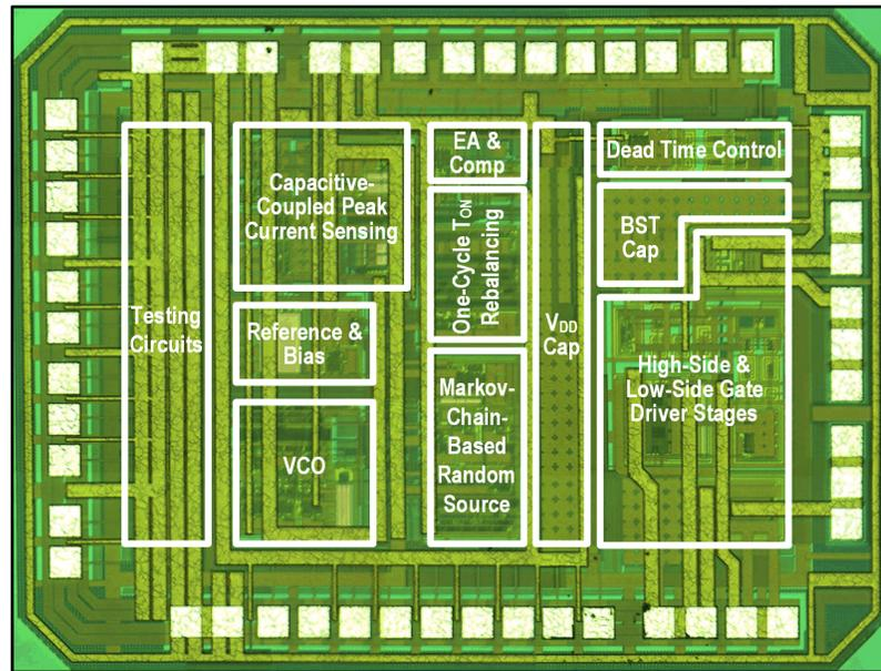
Figure 4.13. Chip micrograph.
