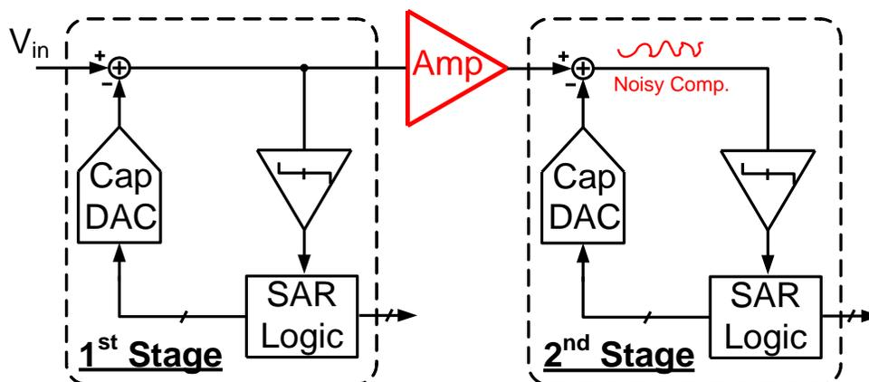
Figure 4.1. Block diagram of pipelined SAR ADC
