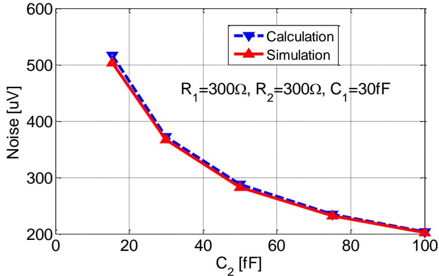
Figure 2.4. Simulated  $kT/C$  noise and the calculated  $kT/C$  noise
