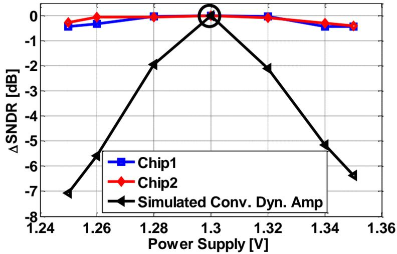
Figure 4.28. Measured SNDR versus the supply voltage
