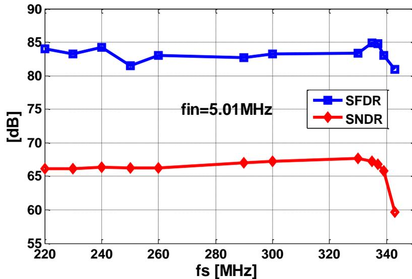
Figure 4.26. Measured SNDR and SFDR vs. sample rate.
