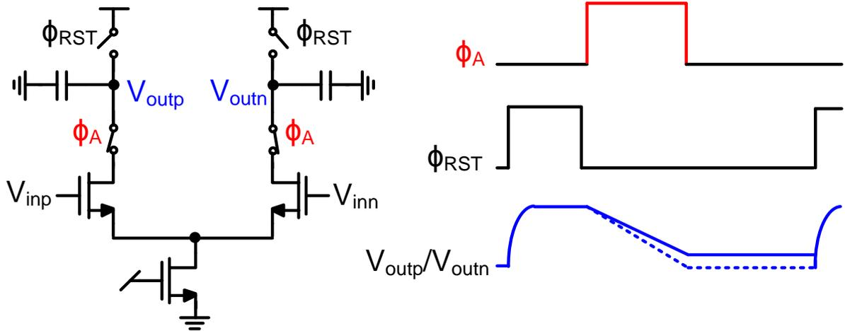
Figure 4.7. Schematic and operation waveforms of open-loop dynamic amplifier
