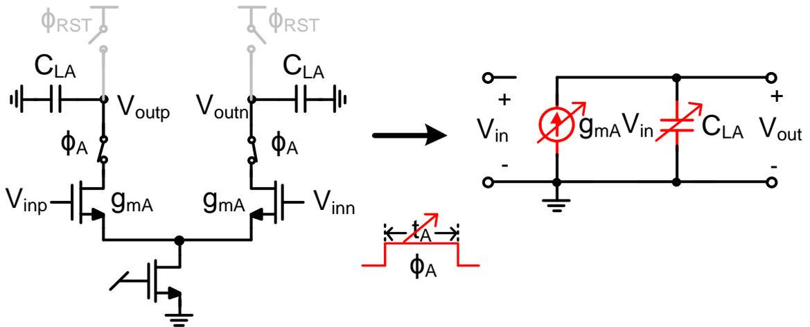
Figure 4.8. Circuit model for open-loop dynamic amplifier
