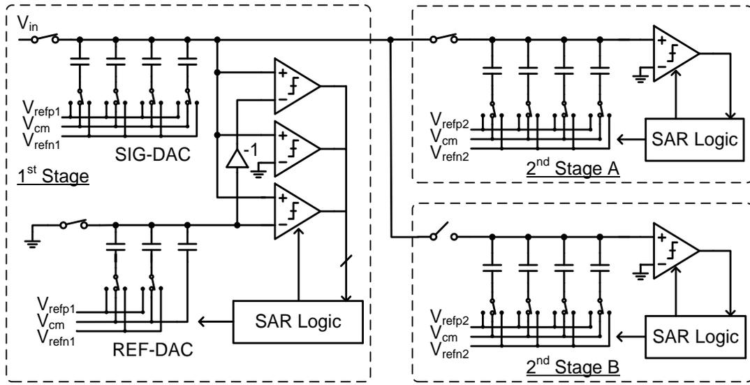
Figure 3.1. Architecture of the 2b-1b/cycle two-step SAR ADC with passive residue transfer(a single-ended version is shown for simplicity)
