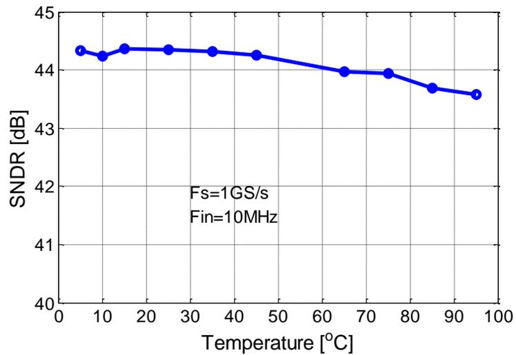
Figure 3.15. Measured SNDR vs. ambient temperature
