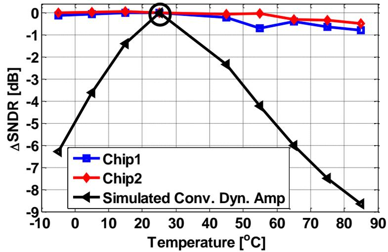
Figure 4.30. Measured SNDR versus temperature
