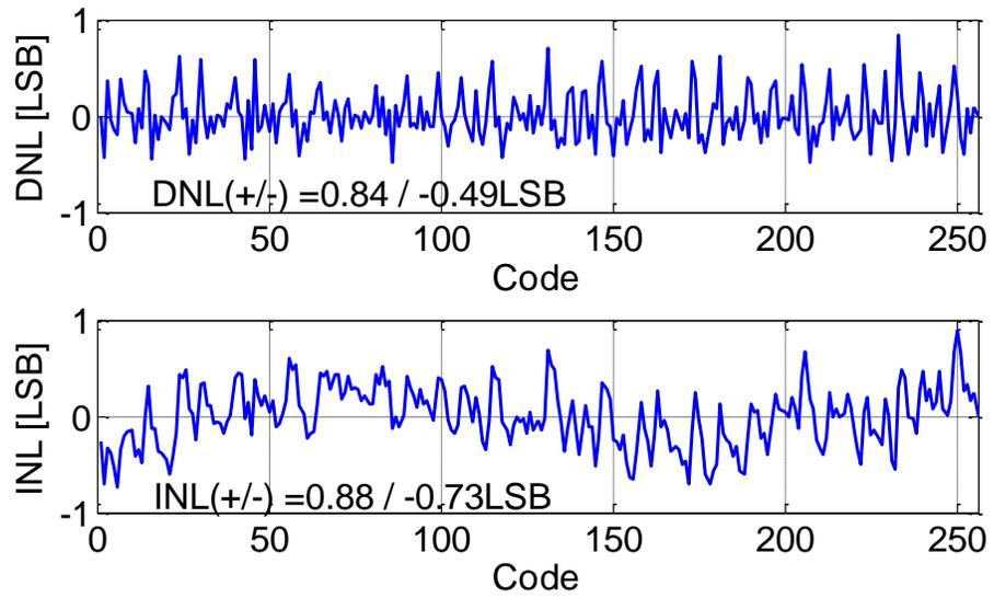
Figure 3.10. Measured DNL and INL profiles
