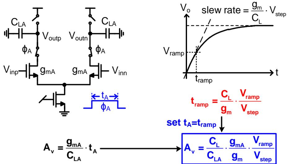
Figure 4.11. Overall concept of PVT stabilization technique
