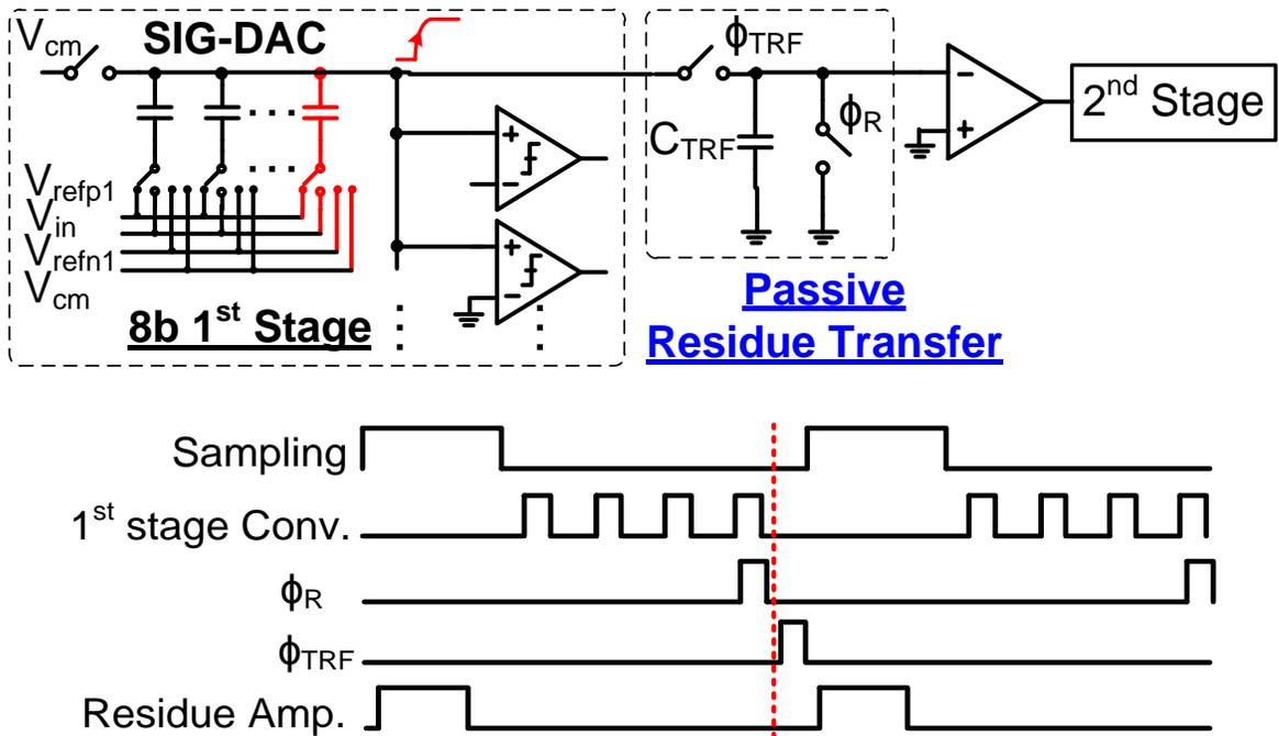
Figure 4.19. Schematic and timing diagram of passive residue transfer
