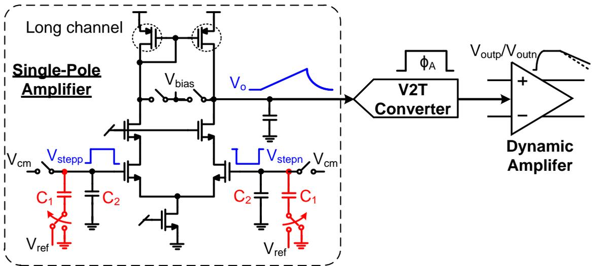
Figure 4.13. Circuit schematic of single-pole amplifier
