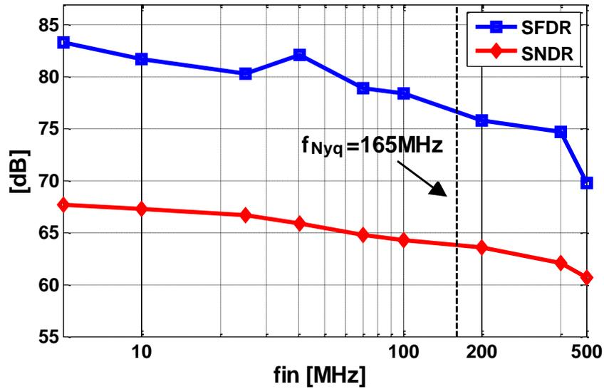
Figure 4.25. Measured SNDR and SFDR vs. input frequency
