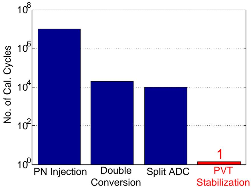
Figure 4.9. Long convergence time of digital background calibration
