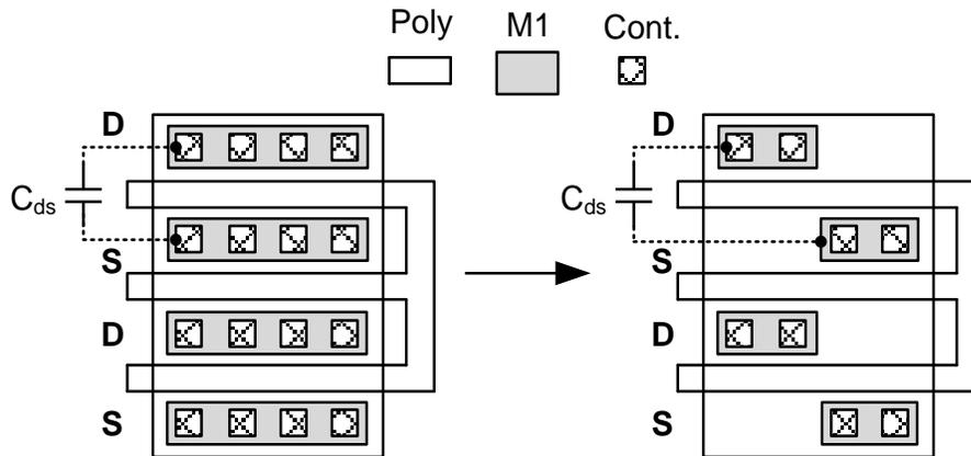
Figure 3.6. Layout of transfer switch with small drain-source capacitance
