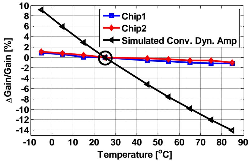
Figure 4.29. Measured residue gain versus temperature
