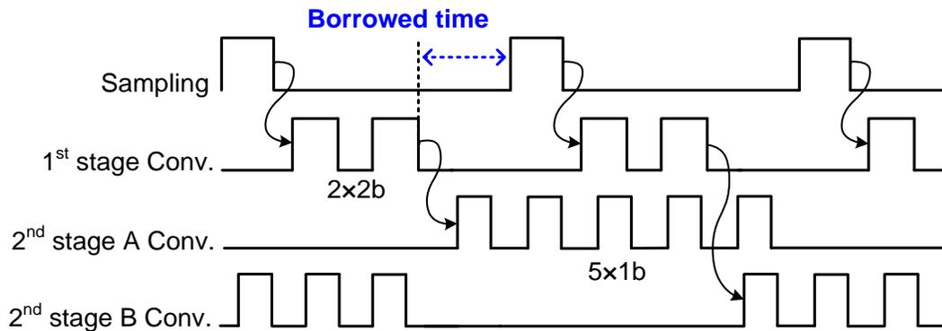
Figure 3.3. Timing diagram of the second resolution partition:  $2 \times 2b$  for the first stage and  $5 \times 1b$  for the second stage
