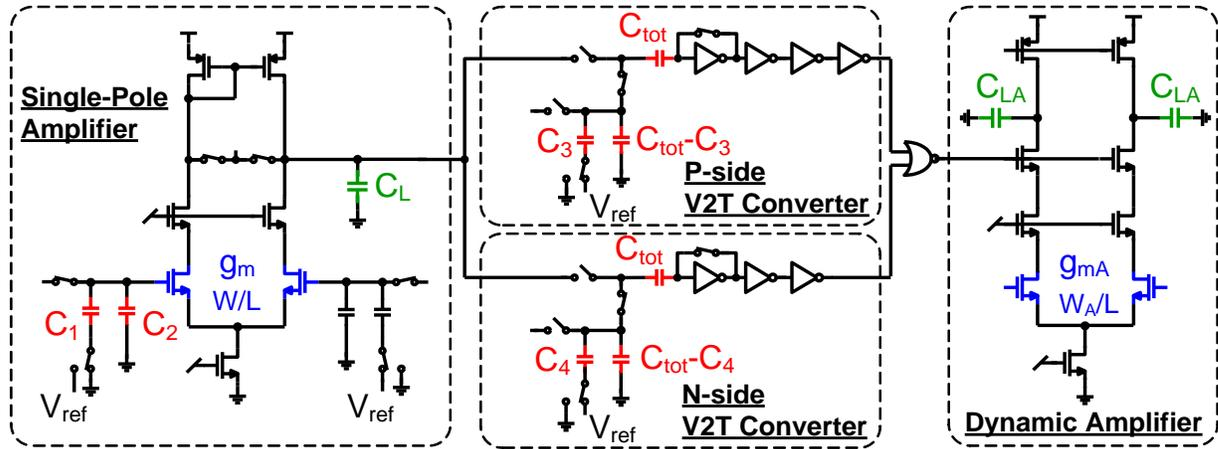
Figure 4.16. Overall schematic of PVT-stabilized dynamic amplifier
