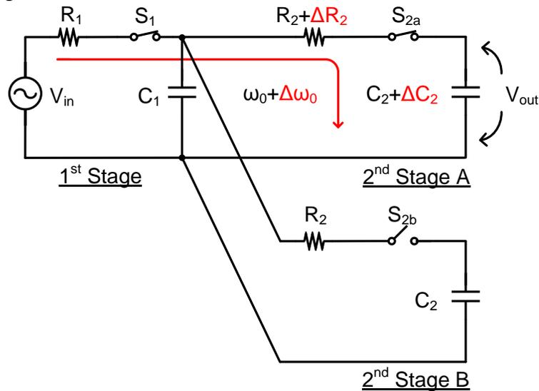
Figure 2.5. Bandwidth mismatch of the sampling network with non-attenuated passive residue transfer
