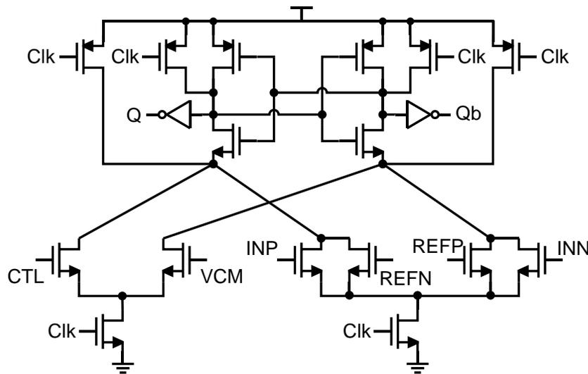
Figure 3.7. Dynamic comparator with an extra input pair for offset calibration
