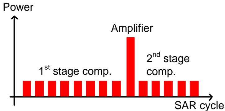
Figure 4.3. Power consumption of pipelined SAR ADC with residue amplifier
