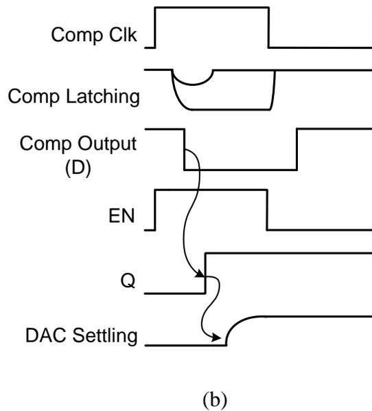
Figure 3.8. (a) Schematic of the dynamic register and (b) Timing diagram of the dynamic register
