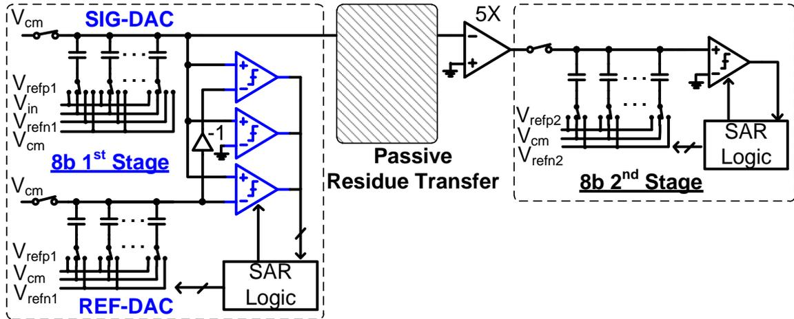
Figure 4.17. Schematic of the prototype pipelined SAR ADC
