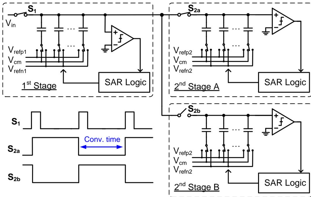
Figure 2.2. Schematic and timing diagram of non-attenuated passive residue transfer
