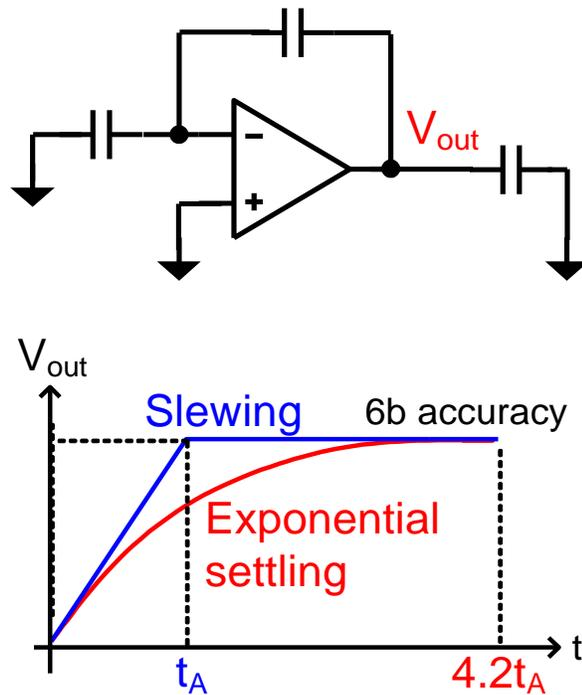
Figure 4.4. Opamp-based residue amplifier and its exponential settling curve
