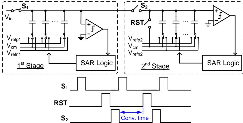
Figure 2.1. Schematic and timing diagram of attenuated passive residue transfer
