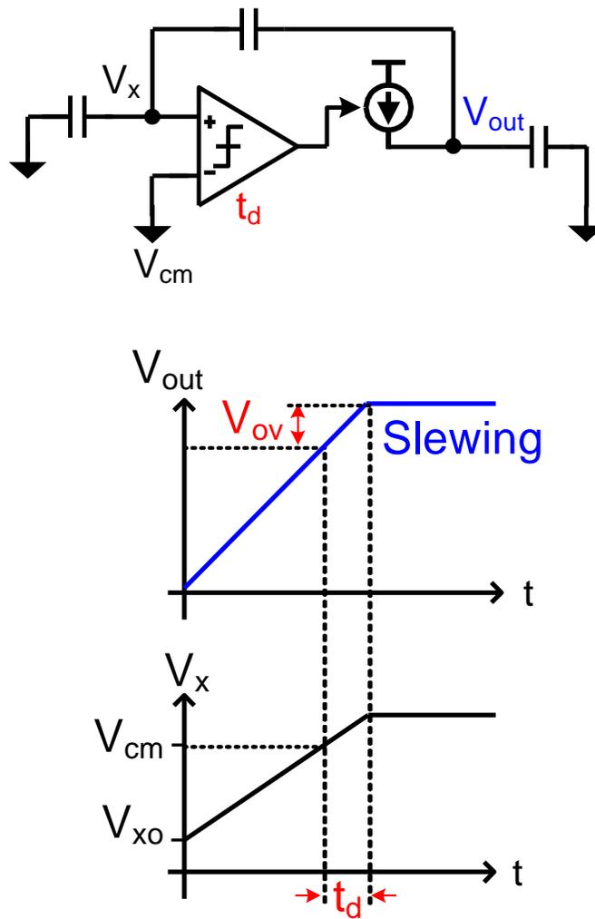
Figure 4.5. Comparator-based residue amplifier and its overshoot problem
