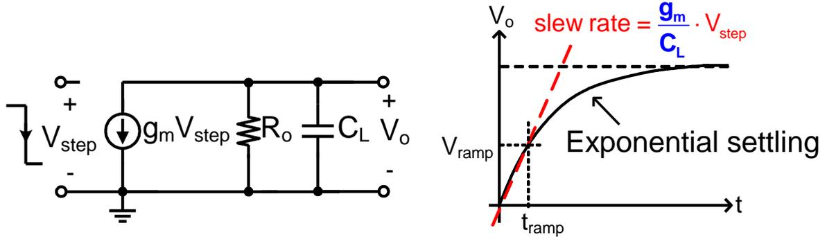
Figure 4.10. The step response of single-pole amplifier
