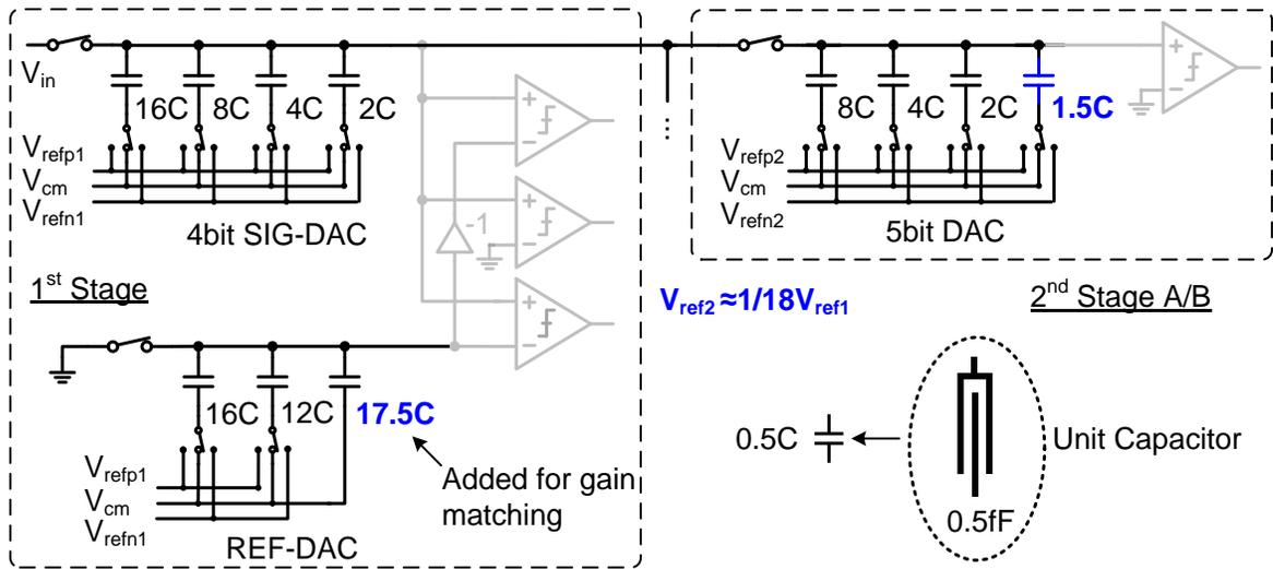
Figure 3.4. Schematic of capacitive DACs in the prototype ADC
