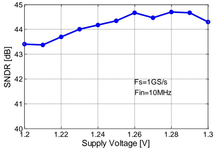
Figure 3.14. Measured SNDR vs. supply voltage
