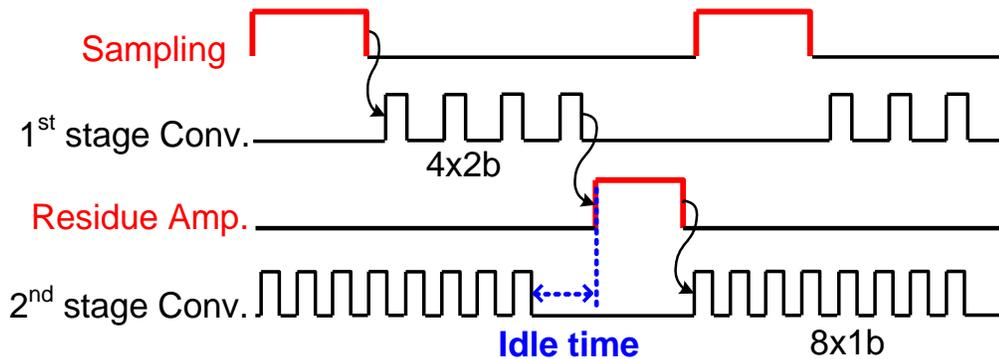
Figure 4.18. Timing diagram of conventional pipelined SAR ADC without passive residue transfer
