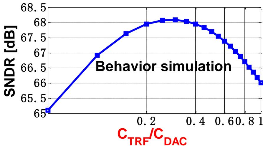
Figure 4.20. Simulated SNR versus  $C_{TRF}/C_{DAC}$
