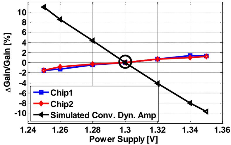
Figure 4.27. Measured residue gain versus the supply voltage
