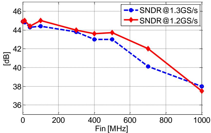
Figure 3.12. Measured SNDR at 1.3 GS/s and 1.2 GS/s vs. input frequency
