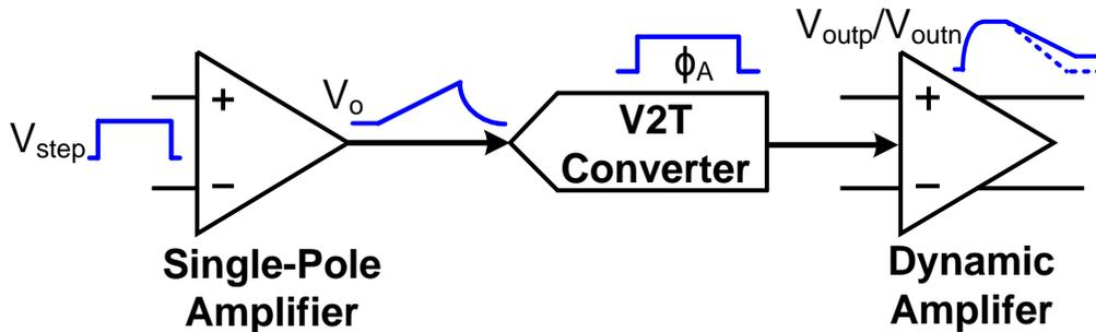
Figure 4.12. Structure of PVT stabilized dynamic amplifier
