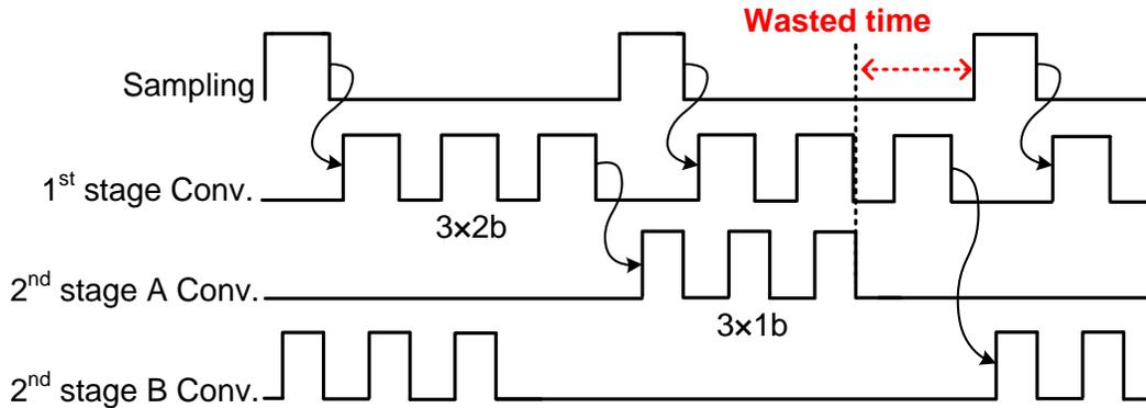
Figure 3.2. Timing diagram of the first resolution partition:  $3 \times 2b$  for the first stage and  $3 \times 1b$  for the second stage
