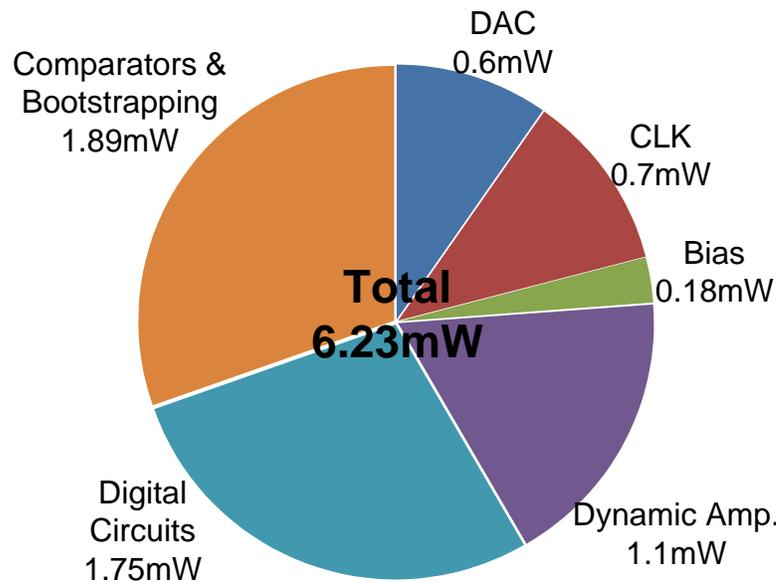
Figure 4.32. Power consumption breakdown of prototype ADC
