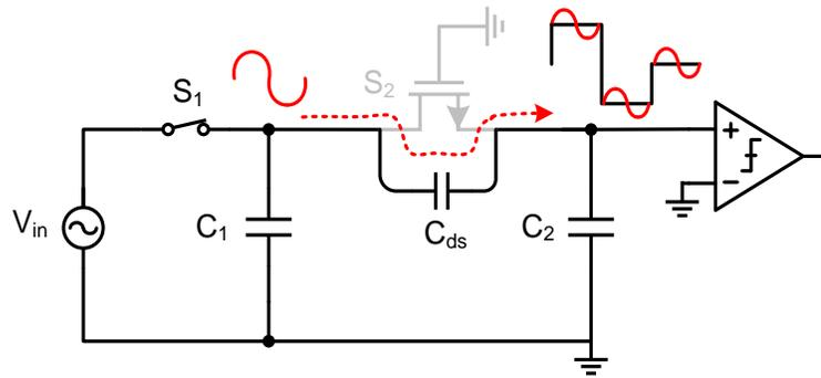
Figure 3.5. Signal feed-through caused by the drain-source capacitance of the transfer switch
