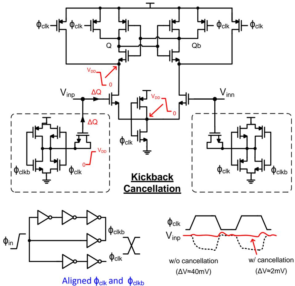
Figure 4.21. Circuit schematic of the dynamic comparator with kickback noise cancellation
