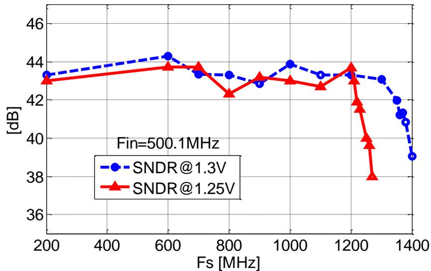
Figure 3.13. Measured SNDR at 1.3 V and 1.25 V supplies vs. sampling frequency
