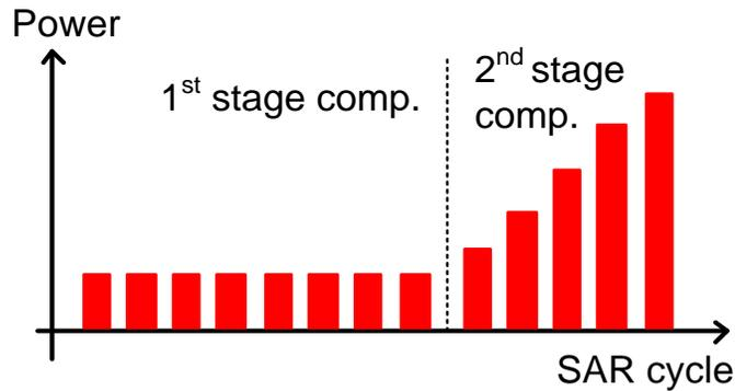
Figure 4.2. Power consumption of pipelined SAR ADC with passive residue transfer
