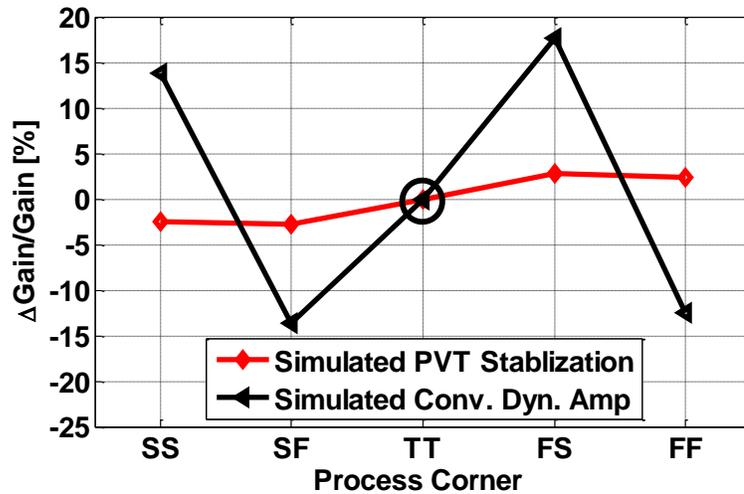
Figure 4.31. Simulated residue versus process corner
