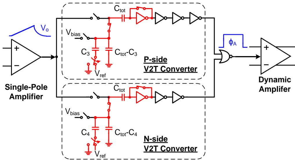
Figure 4.14. Circuit schematic of voltage to time converters
