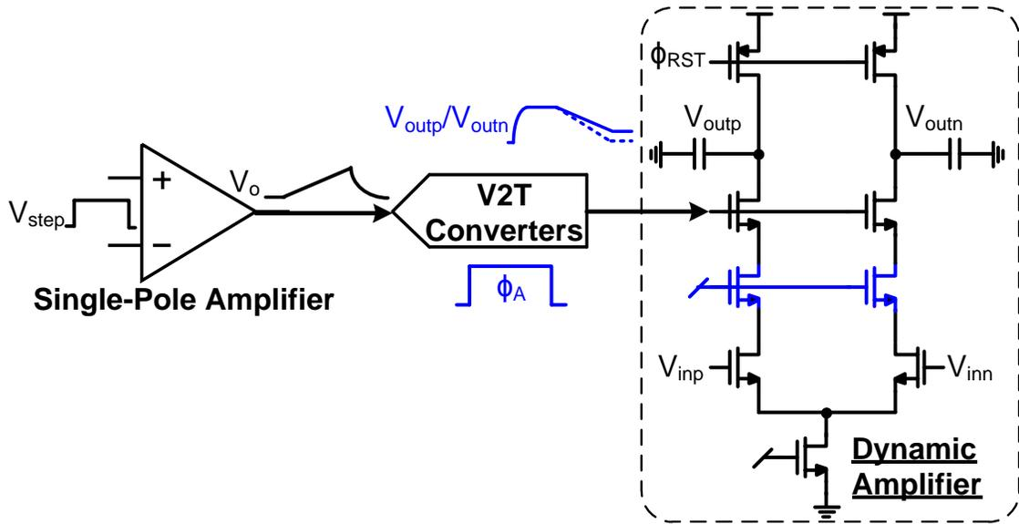
Figure 4.15. Circuit schematic of dynamic amplifier
