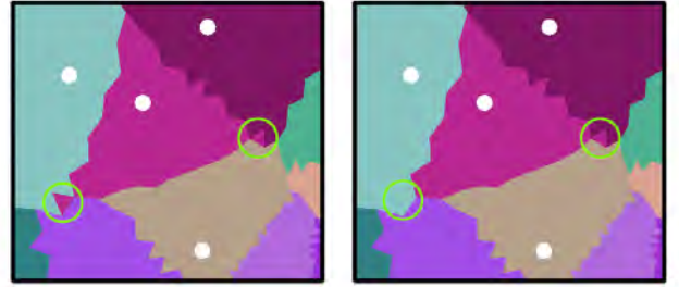
Fig. 7. Left: the accurate discrete Voronoi diagram; Right: the mesh flooding result. Two disconnected triangles are marked by circles.
