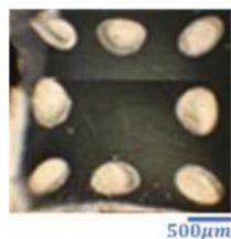
Fig. 3. Composite image of fabricated waveguide cross section.
