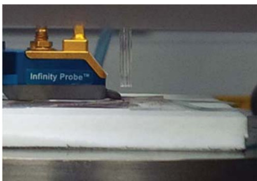
Fig. 7. Side view showing waveguide is not directly touching the microstrip antenna and substrate. The patch radiates above the substrate and the field is coupled to the waveguide.
